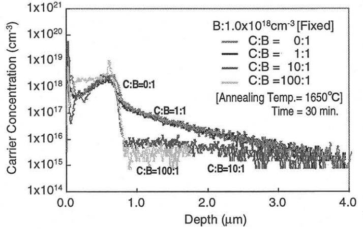
Fig.2 SIMS profile of B implanted 4H-SiC showing a long diffusion tail after annealing at 1650°C for 30min. in Ar ambient. The C/B sequential implantation limits the B diffusion in 4H-SiC.
