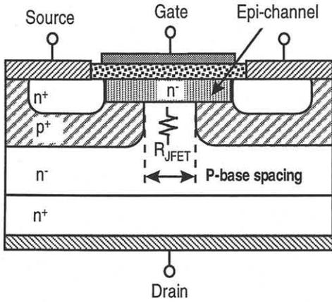
Fig.1 Schematic structure of accumulation-mode planar epi-channel field effect transistor (ECFET).
