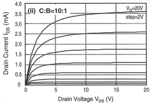
Fig.4  $I_{DS}$ - $V_{DS}$  characteristics of accumulation-mode planar 4H-SiC ECFET with (i). B implanted p-base region, and (ii). C/B sequentially implanted p-base region. The effectiveness of C/B sequential implantation in suppressing the JFET pinch effect is clearly visible from the 3-4 fold increase in  $I_{DS}$  of planar ECFET (P-base spacing= 3 $\mu\text{m}$ ).
