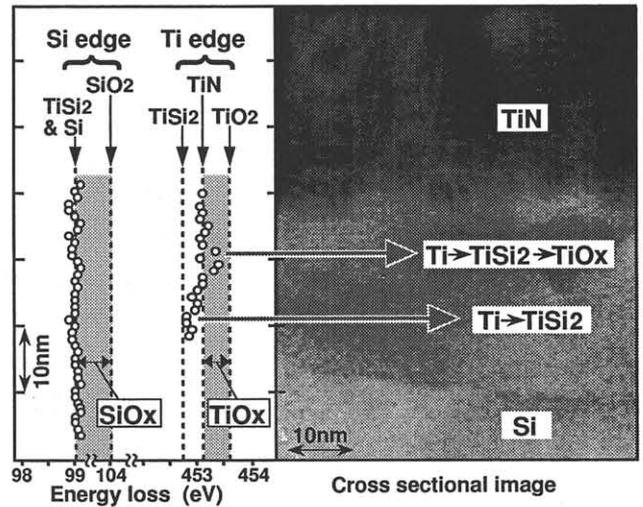
Fig. 4 TEM image and line profiles of core-loss edge energies at a contact bottom with high resistivity ( $k\Omega$ ). Chemical shifts of Ti reveal that Ti is partially oxidized.
