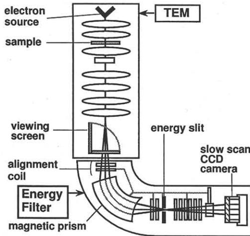
Fig. 2 Schematic diagram of TEM-EELS. Spatially-resolved EELS provides plural spectra at different points simultaneously.
