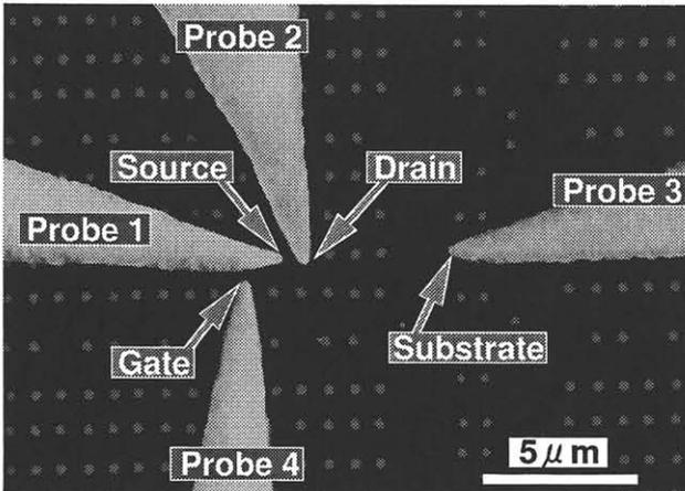
Probes on a  $0.2\mu\text{m}$  Processor
