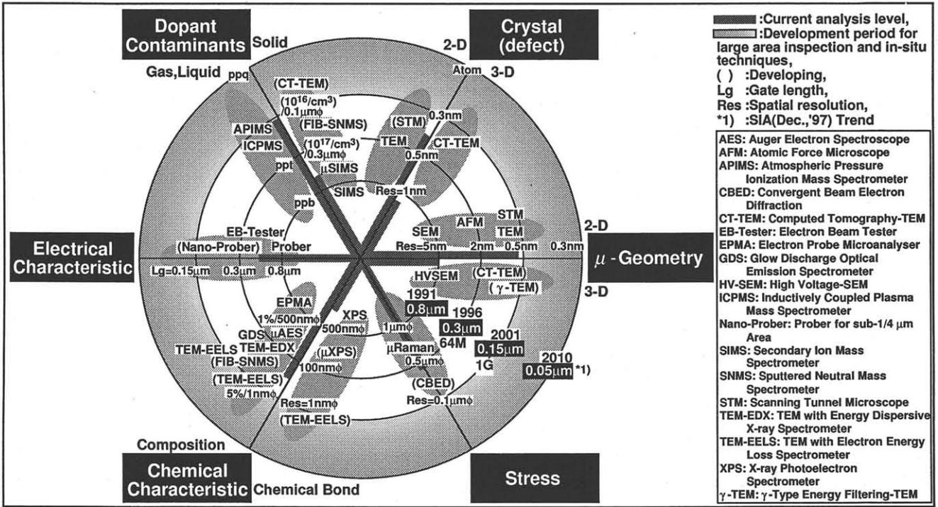
Fig. 1 Current status and future trend of analytical instruments for failure analyses.
