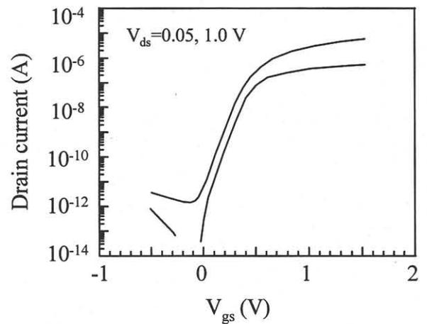
Figure 5: Transfer characteristics for fabricated double-gate MOSFET [9].  $L_{\text{gate}} = 30 \text{ nm}$ ;  $T_{\text{Si}} = 20 \text{ nm}$ .
