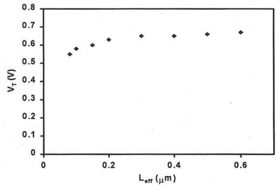
Figure 4: Threshold voltage roll-off for fabricated thin-body MOSFETs [6]. Channel (20 nm thick) was formed by deposition of a-Si and subsequent lateral epitaxial crystallization.
