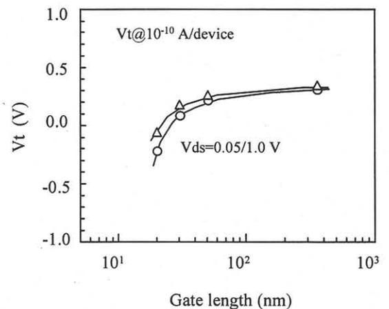
Figure 6: Threshold voltage roll-off for fabricated double-gate MOSFETs [9].  $T_{\text{Si}} = 20 \text{ nm}$ .
