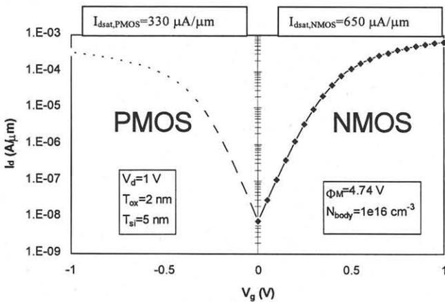
Figure 3: Simulated transfer characteristics for optimized 25 nm gate-length thin-body MOSFETs [5].
