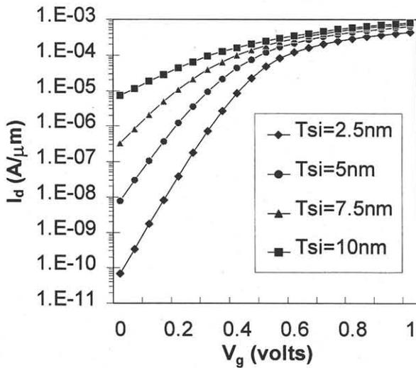
Figure 2: Simulated 25 nm gate-length thin-body MOSFET transfer characteristics for various body thicknesses [5].  $N_{\text{body}} = 10^{16} \text{ cm}^{-3}$ ;  $T_{\text{ox}} = 2 \text{ nm}$ ;  $\Phi_M = 4.74 \text{ V}$ .
