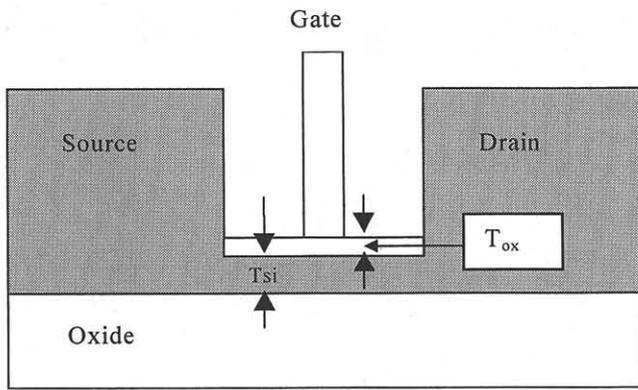
Figure 1: Thin-body MOSFET structure.
