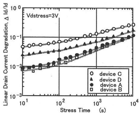
Fig. 1 Degradation of linear drain current. The extension dose and pocket dose were varied as parameters.
