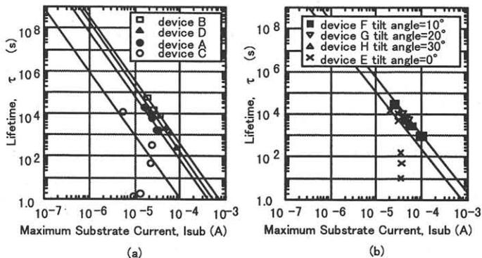
Fig. 4 Dependence of hot carrier lifetime on the maximum substrate current.
