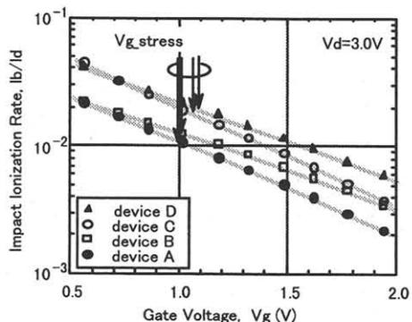
Fig. 2 Impact ionization rate of devices shown in Fig. 1.
