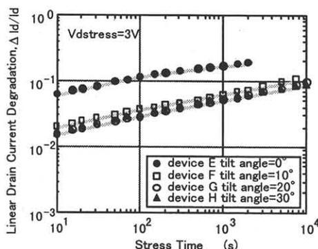
Fig. 3 Degradation of linear drain current. The extension implantation angle was changed as a parameter.
