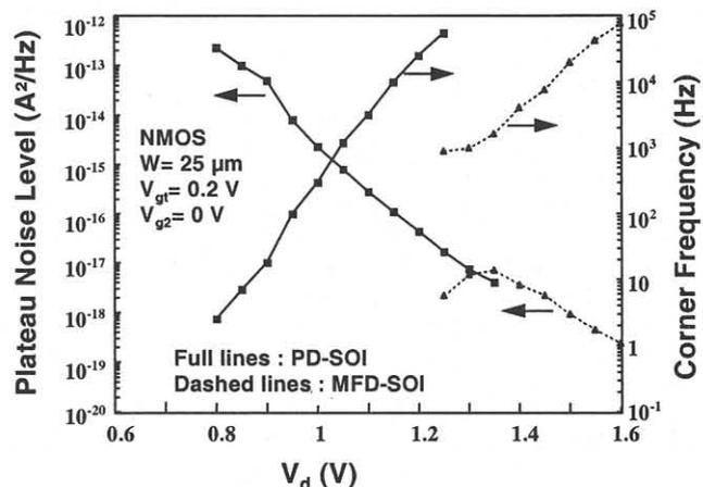
Figure 4. Drain bias dependence of the plateau noise level and the corner frequency for  $0.25\mu\text{m}$  PD device with floating body (full lines) and  $1\mu\text{m}$  MFD device (dashed lines).
