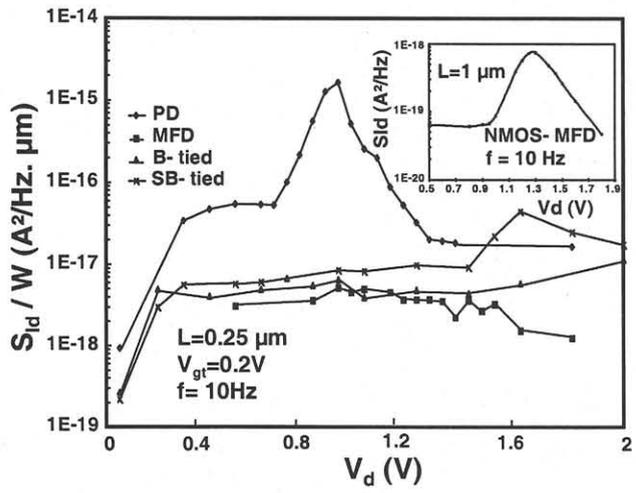
Figure 2. Drain current noise spectral density, normalized by the width  $W$ , at the frequency  $f=10$  Hz, for the four different architectures, versus drain bias. The inset shows the drain current spectral density versus  $V_d$  for the MFD device at  $L=1\mu\text{m}$ .
