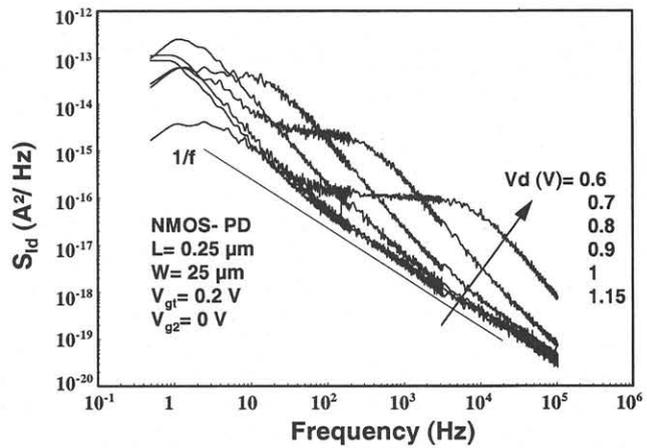
Figure 3. Drain current spectral density versus frequency for the  $0.25\mu\text{m}$  PD device (floating body), at different drain voltages.
