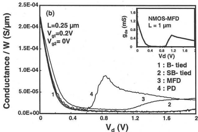
Figure 1. Output drain current (a) and conductance (b), normalized by the width  $W$ , versus drain bias for different layouts. The gate voltage is  $V_{gt} = 0.2$  V. The insets show the drain current and the output conductance for  $1\mu\text{m}$  MFD SOI device.
