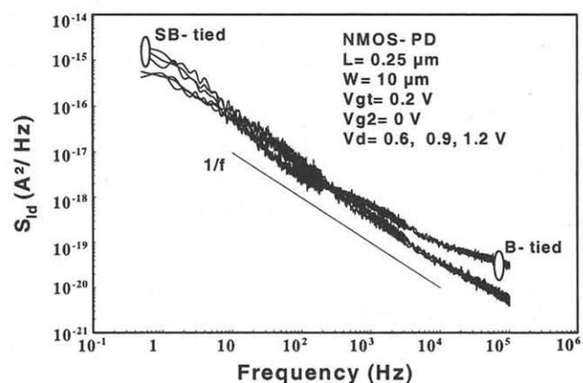
Figure 5. Drain current spectral density versus frequency for body tied and source-body tied devices, at different drain voltages.  $W/L=10/0.25\mu\text{m}$ , and  $V_{gt}=0.2$  V
