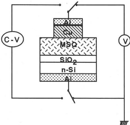
Fig.1. Sample capacitor structure and measurement setup. Al(100nm)/Cu (500nm)/MSQ(4000nm)/SiO<sub>2</sub>(100nm)/Si.
