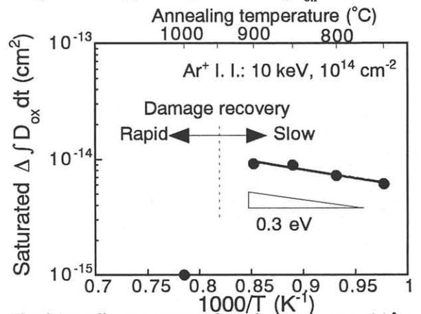
Fig. 6 Annealing temperature dependence on saturated  $\Delta f D_{ox} dt$ .
