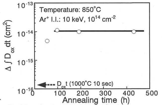
Fig. 5 Annealing time dependence on  $\Delta f D_{ox} dt$ .
