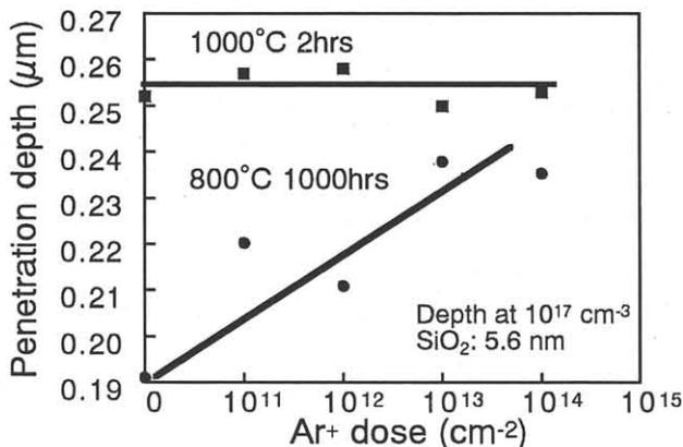
Fig. 3 Ar<sup>+</sup> dosage dependence on penetration depth.
