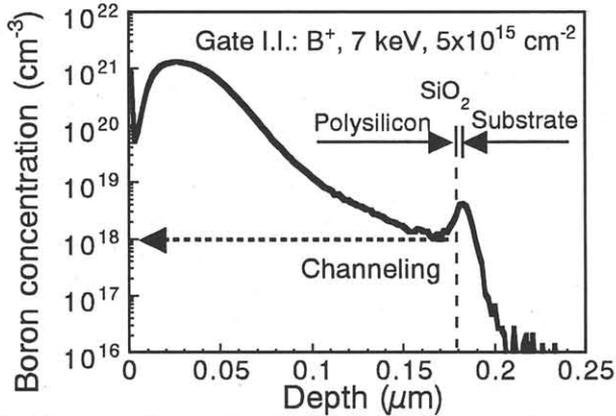
Fig. 1 Boron profile in gate poly-Si just after B<sup>+</sup> ion implantation.
