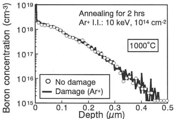
Fig. 4 Boron profile in substrate after annealing at 1000°C for 2 h.
