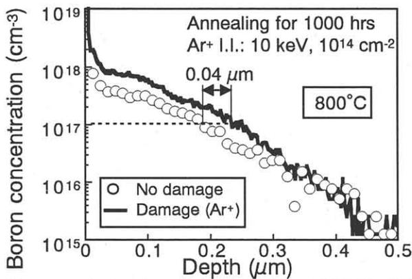
Fig. 2 Boron profile in substrate after annealing at 800°C for 1000 h.
