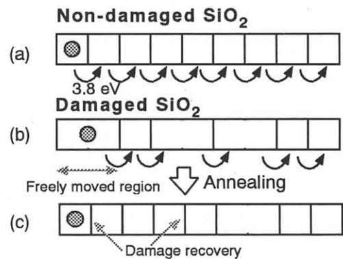
Fig. 7 A model of enhanced boron diffusion caused by ion implantation damage.
