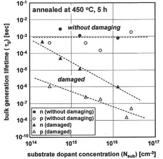
Fig. 4 Bulk generation lifetime ( $\tau_g$ ) of "damaged MOS capacitor" plotted as a function of substrate dopant concentration.
