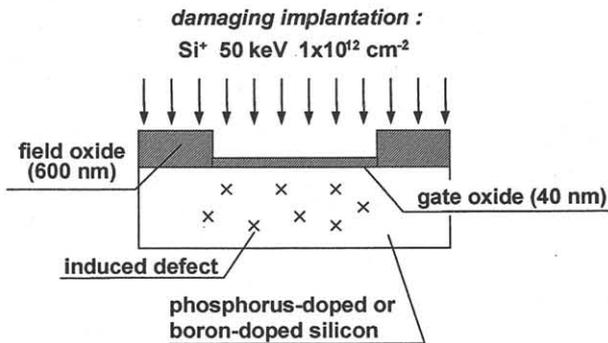
Fig. 3 Schematic picture of special sample named "damaged MOS capacitor".
