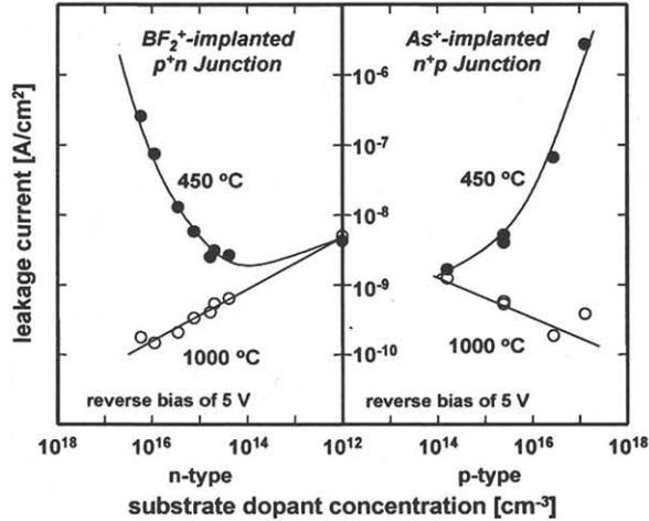
Fig. 1 Leakage current density at reverse bias of 5V plotted as a function of substrate concentration ( $N_{sub}$ ) for both  $As^+$ -implanted  $n^+p$  junction and  $BF_2^+$ -implanted  $p^+n$  junction annealed at 450°C and 1000°C.
