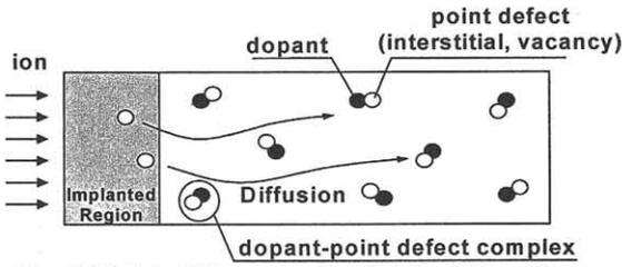
Fig. 2 Model of "dopant-induced defect" formation.
