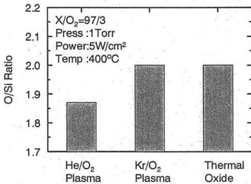
Fig.3 O/Si ratio in silicon oxide grown by Kr/O<sub>2</sub> and He/O<sub>2</sub> mixed high-density plasma at a temperature of 400 °C
