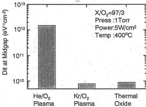
Fig.4 Interface trap density versus growth condition
