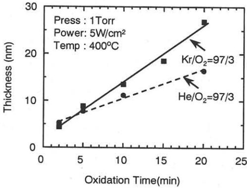
Fig.2 Oxidation rate of Kr/O<sub>2</sub> and He/O<sub>2</sub> mixed high-density plasma at a temperature of 400 °C
