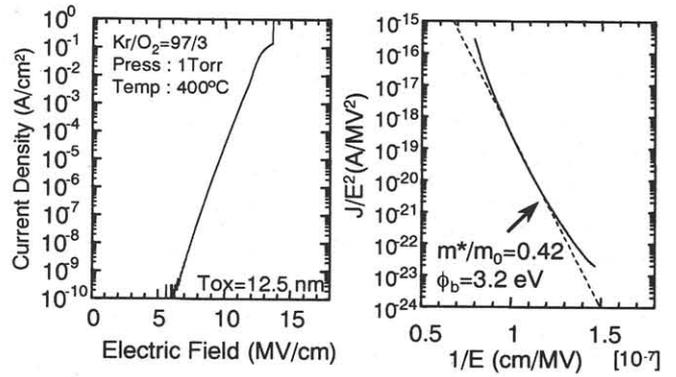
Fig.6 J-E curve and Fowler-Nordheim plot of silicon oxide with thickness of 12.5 nm grown by Kr/O<sub>2</sub> plasma
