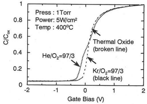
Fig.5 C-V curves of silicon oxide grown by Kr/O<sub>2</sub> and He/O<sub>2</sub>
