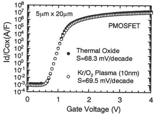
Fig.7 Subthreshold characteristic of silicon oxide grown by Kr/O<sub>2</sub> at 400 °C and thermally grown silicon oxide
