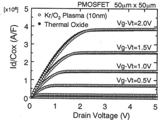
Fig.8 Vd-Id characteristics of silicon oxide
