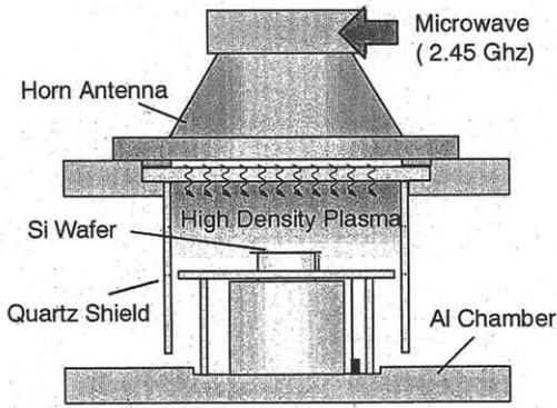
Fig.1 Schematic of microwave-excitation plasma process equipment
