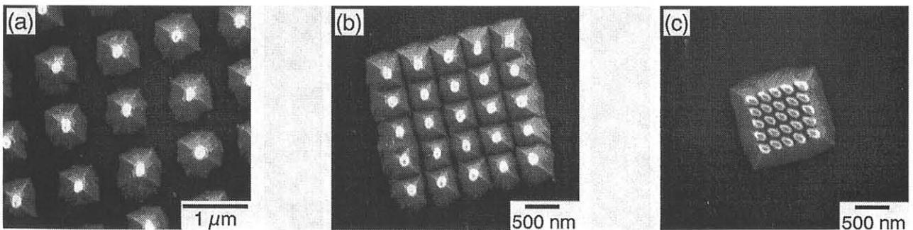
Fig.2 SEM images of nanopyramid arrays processed by the dot exposure of 60 keV Si FIB at a dose of  $5 \times 10^{14} \text{ cm}^{-2}$  with interval of (a)  $1 \mu\text{m}$ , (b)  $500 \text{ nm}$  and (c)  $200 \text{ nm}$ .
