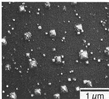
Fig.3 SEM images of nanopyramid arrays processed by the dot exposure of 60 keV Si FIB at a dose of  $5 \times 10^{13} \text{ cm}^{-2}$ .
