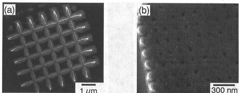
Fig.4 SEM images of pyramidal etchpit arrays processed by the line exposure of 60 keV Si FIB at a dose of  $5 \times 10^{14} \text{ cm}^{-2}$  with interval of (a)  $1 \mu\text{m}$  and (b)  $150 \text{ nm}$ .
