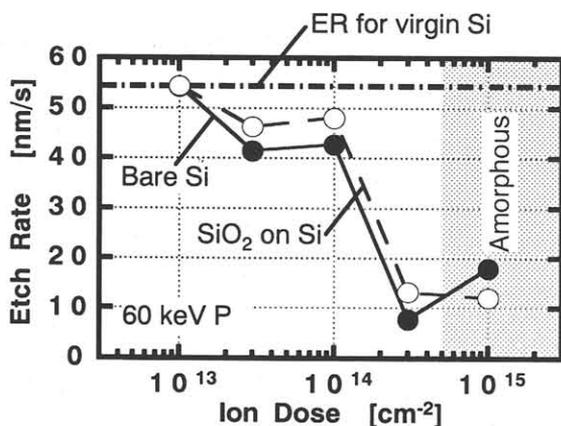
Fig.5 Dependence of etch rate of Si by hydrazine on the ion dose.
