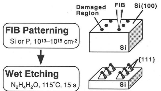
Fig.1 Nanopyramid array fabrication process flow
