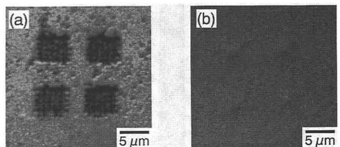
Fig.6 Optical micrograph of pyramidal etchpit arrays (a) after annealing for recrystallization in  $\text{N}_2$  at  $850^\circ\text{C}$  for 2 min and (b) after the subsequent dipping in hydrazine solution for 15 s at  $115^\circ\text{C}$ .
