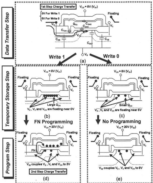
Fig. 3 Three-step programming procedure: (a) the 1st step of data transfer: Different bitline voltages invert different channel charges. (b)(c) the 2nd step of temporary storage: Cells which have stored data in the channel have to wait for data-transfer of other cells. FN tunneling is inhibited. (d)(e) the 3rd step of programming: Charges are tunneled into the floating gate if abundant charges existing in the channel inversion. Otherwise, no tunneling occurs.
