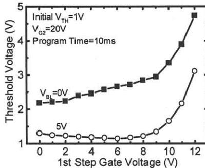
Fig. 5 Threshold voltage vs. 1st step gate voltage ( $V_{G1}$ ) for programming and non-programming.
