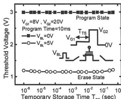
Fig. 8 Programmed threshold voltage vs. temporary storage time ( $T_{TS}$ ).
