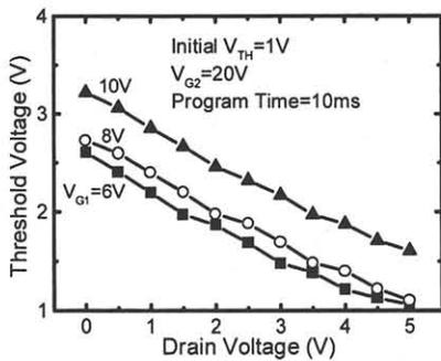
Fig. 4 Threshold voltage vs. drain voltage for different 1st step gate voltage ( $V_{G1}$ ).
