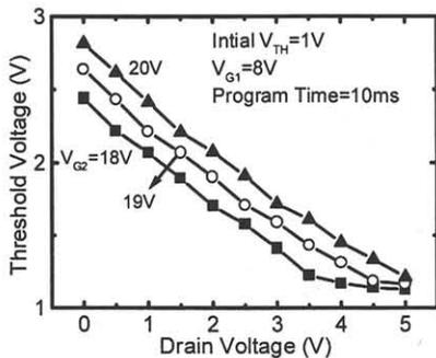
Fig. 7 Threshold voltage vs. drain voltage for different 2nd step gate voltage ( $V_{G2}$ ).
