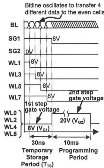
Fig. 2 Timing diagram of high-speed multiple-wordline programming. During temporary storage period, even cells function as data latches. After latching, even cells are programmed simultaneously.
