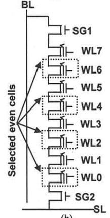
Fig. 1 (a) Cell cross section, (b) NAND array is divided into even/odd cells.
