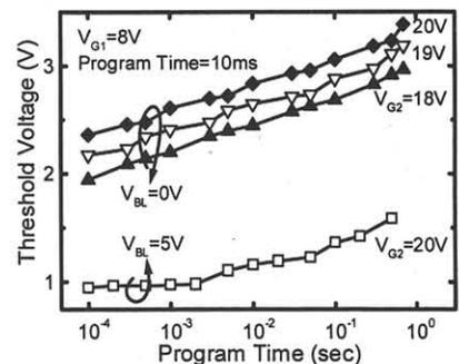
Fig. 6 Programming trend for different programming and non-programming.
