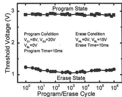
Fig. 9 Endurance characteristics. No window closing is observed.
