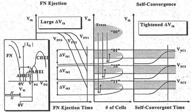
Fig. 2  $V_{th}$  dispersion controlling scheme for multi-level AND-type Flash memory
