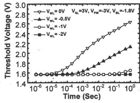
Fig. 11 Bit-line disturbance for "11" state vs. word-line inhibition voltage
