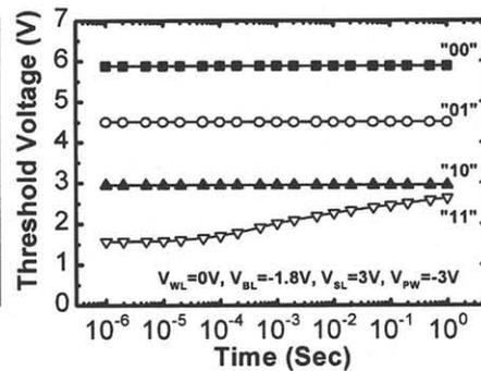
Fig. 10 Bit-line disturbance during self-convergent operation
