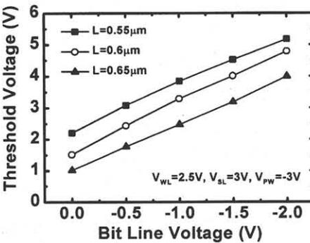
Fig. 6 Convergent threshold voltage vs. bit-line voltage
