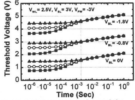
Fig. 5 Self-convergent characteristics with different bit-line voltages
