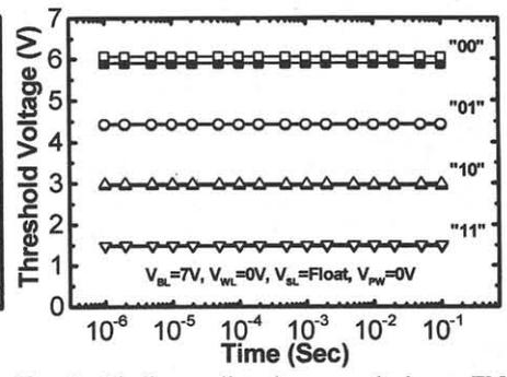
Fig. 8 Bit-line disturbance during FN program for fresh/after-cycled cell (solid/open symbol)
