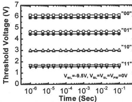
Fig. 9 Word-line disturbance during FN program for fresh/after-cycled cell (solid/open symbol)
