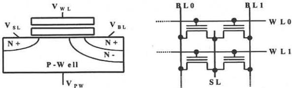
Fig. 1 Cell structure and array architecture
