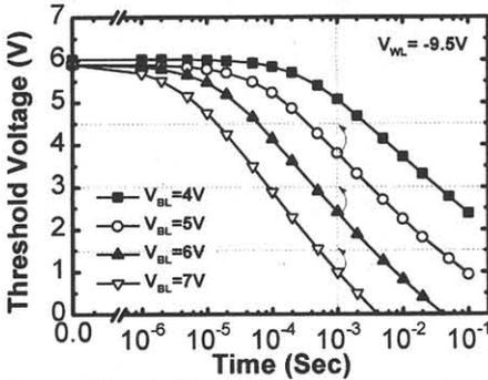
Fig. 3 Threshold voltage vs. programming time during FN ejection
