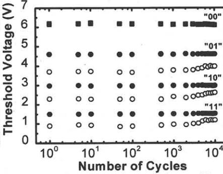
Fig. 7 Endurance characteristics with/without (solid/open symbol) self-convergent operation
