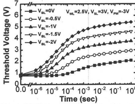
Fig. 4 CHISEL operation with different bit-line voltages
