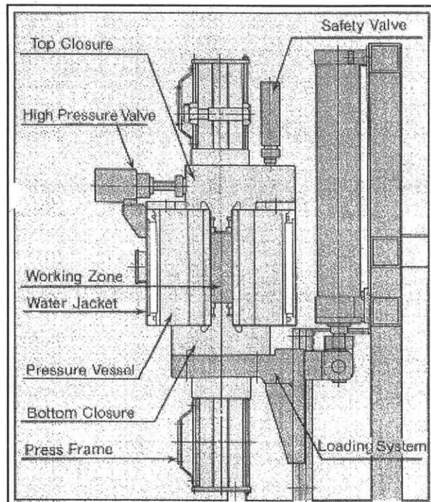
Fig. 2 Schematic cross sectional view of the high pressure furnace.
