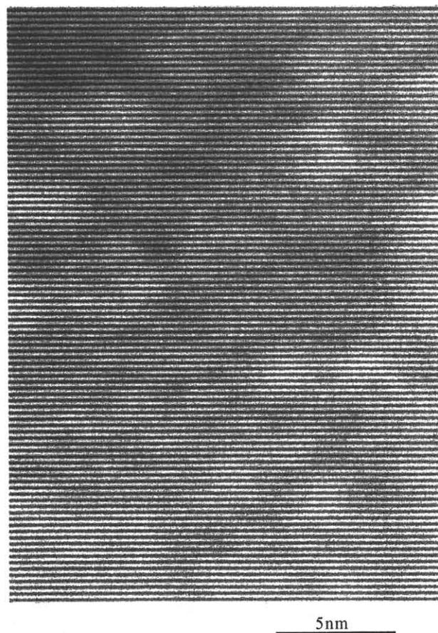
Fig. 4 Cross sectional TEM image of the GaN single crystal.
