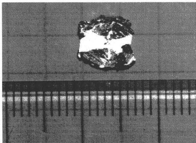
Fig. 3 GaN single crystal grown by the pressure-controlled high pressure solution growth (PC-SG) method.
