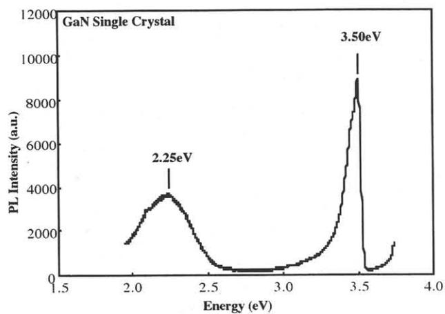
Fig. 5 Photoluminescence spectrum at 4.2 K of the GaN single crystal.
