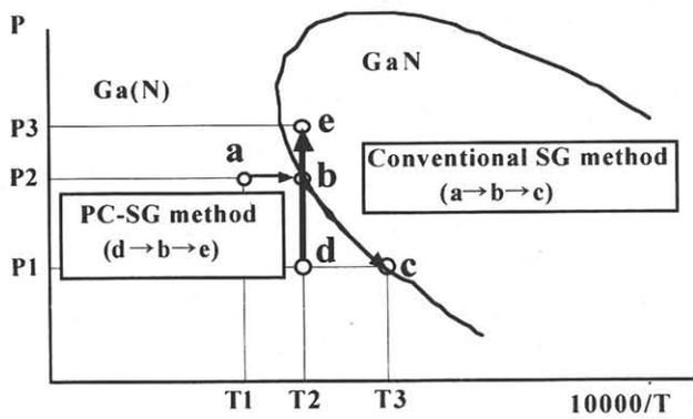
Fig. 1 Schematic P-T diagram of GaN.
