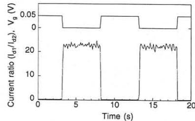
Fig. 7. Switching operation for an input top-gate voltage ( $V_g$ ) with an amplitude of 50 mV (between 0 and 50 mV). Voltage to the side gates, 1 and 2 are set to be 0 V. Current ratio is defined by  $I_{a1}/I_{a2}$ , where  $I_{a1}$  and  $I_{a2}$  represent the current flowing into Drain 1 and Drain 2, respectively.
