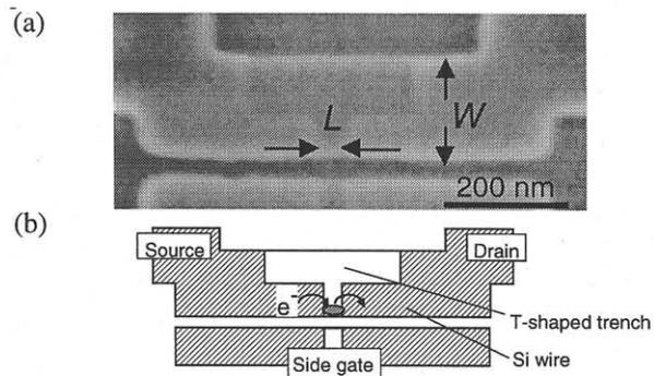
Fig. 3. SEM image (a) and its schematic view (b) of the SET with  $L$  of 30 nm,  $W$  of 160 nm, and the trench depth  $d$  of about 10 nm. The top gate is not shown.
