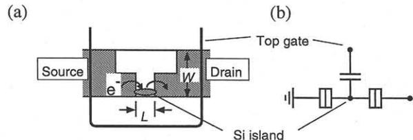
Fig. 2. Top view (a) and equivalent circuit (b) of the SET. Current flows only along the shorter edge, whose length is denoted by  $L$ .
