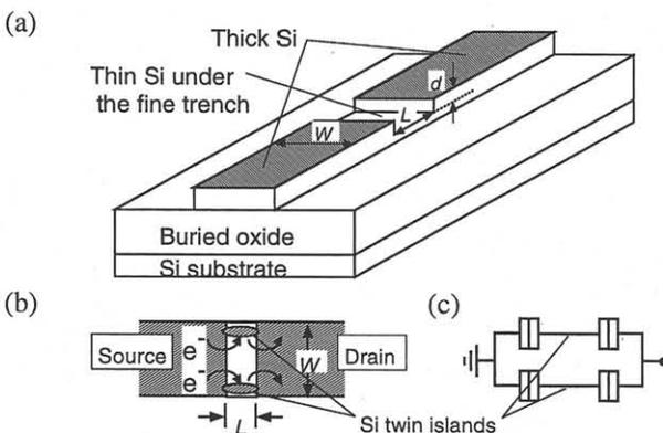
Fig. 1. Basic pre-oxidation Si pattern for V-PADOX (a), and the top view (b) and the equivalent circuit (c) of the pattern after oxidation.  $W$ ,  $L$  and  $d$  represent the wire width, the length of the thin region, and the trench depth, respectively. Since the basic pattern has a rectangular thin region, whose length is defined by  $L$ , twin islands with almost the same size are formed after oxidation [1].
