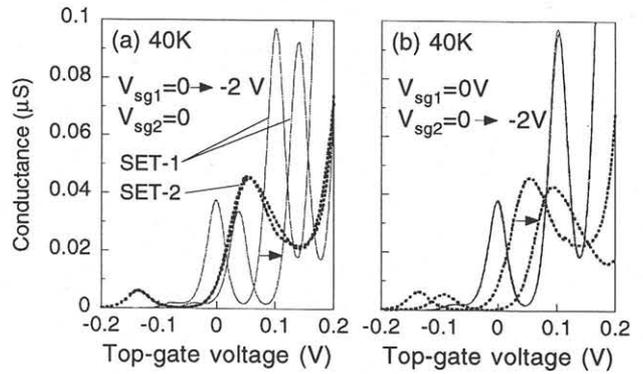
Fig. 6. Conductance characteristics of each SET in the current switching device. Shorter-edge length  $L$  is 30 nm for both SETs. Source-drain voltage was 10 mV for both SETs. In (a), change in  $V_{sg1}$  from 0 to -2 V shifts the conductance curve of SET-1 to the positive direction while that of SET-2 is not shifted. The situation in (b) is converse of that in (a).
