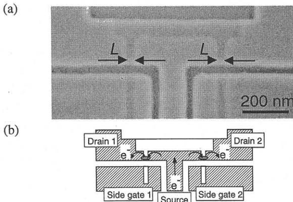
Fig. 5. SEM image of the current-switching device (a) and its schematic view (b). Shorter-edge length  $L$  is 30 nm for both SETs.
