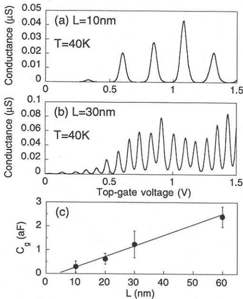
Fig. 4. Conductance characteristics of the SETs with the shorter-edge length  $L$  of 10 (a) and 30 nm (b), and the top-gate capacitance  $C_g$  as a function of  $L$  (c). In (a) and (b), the source-drain voltage was 10 mV, and the voltage to the side gate was 0 V.
