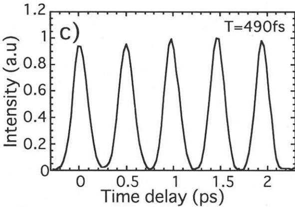
Fig. 1 Phase locked control pulse sequence generated by pulse shaping technique.
