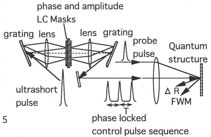
Fig. 2. Experimental setup for the manipulation of coherent exciton in single and coupled quantum wells. The phase locked control pulse sequence is generated by pulse shaping system.
