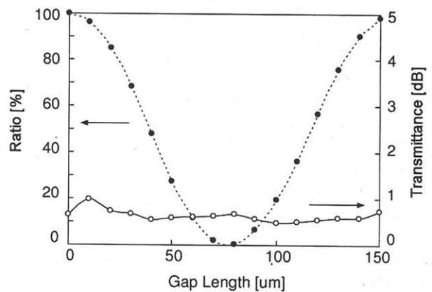
Figure 4: Power splitting ratio and excess loss of MMI coupler fabricated with divided gap design.
