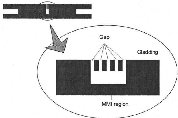
Figure 3: Divided gap design to suppress gap radiation loss.
