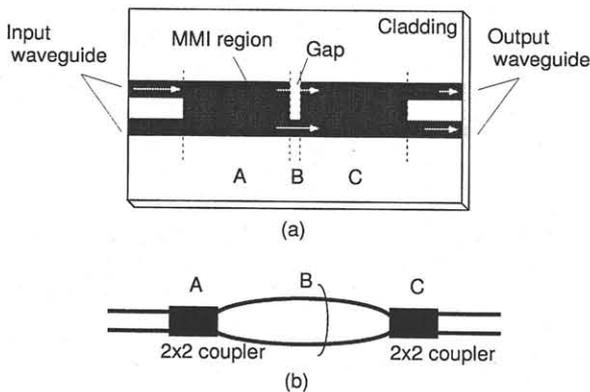
Figure 1: (a) A schematic configuration of our proposed MMI coupler with an arbitrary splitting ratio, (b) A Mach-Zehnder interferometer with the same function as the MMI coupler.
