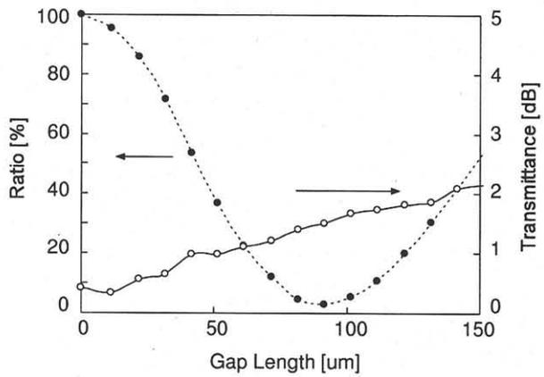
Figure 2: Power splitting ratio and excess loss of MMI coupler fabricated with a single gap.
