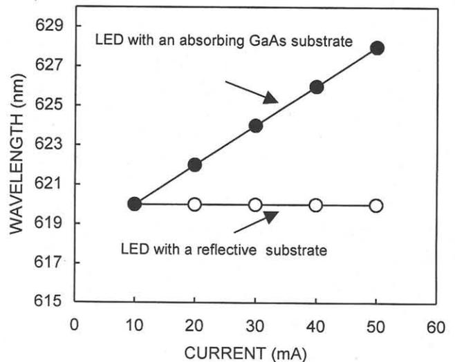
Fig. 4 Peak spectral wavelength as a function of DC drive current for the LEDs with an absorbing GaAs substrate and a reflective substrate.
