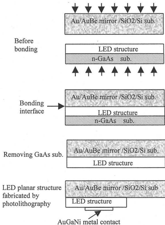
Fig. 1 Wafer bonding process
