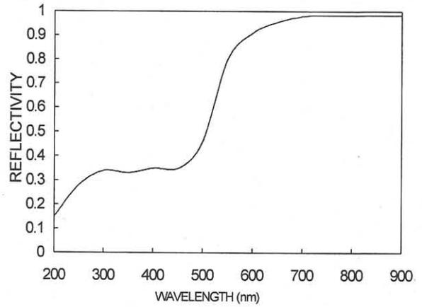
Fig. 2 Reflectance spectrum of the processed Au/AuBe/SiO<sub>2</sub>/Si mirror.
