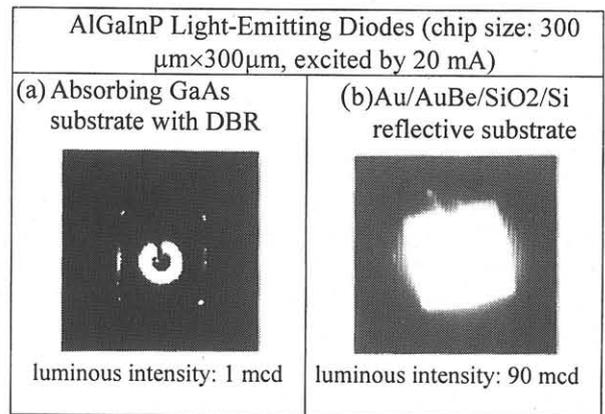
Fig. 3 Photomicrographs of AlGaInP LEDs with (a) a DBR structure on an absorbing GaAs substrate and (b) a bonded substrate under a forward 20-mA injection.
