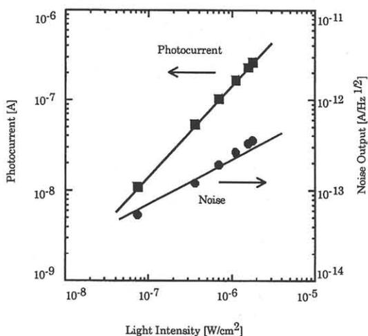
Fig.3 Dependence of signal and noise outputs on incident light intensity.
