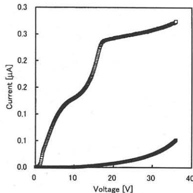
Fig.2 The photocurrent characteristics of the staircase photodiode film with one band discontinuity
