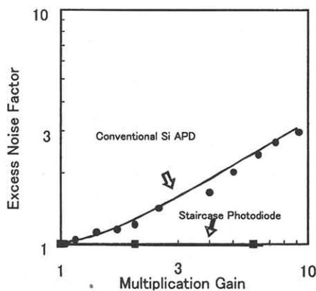
Fig.5 Comparison between excess noise factor of the conventional Si APD and of the a-Si/a-SiC staircase photodiode films.
