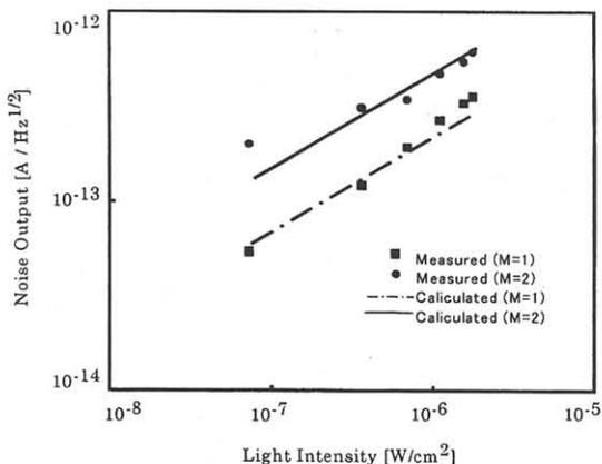
Fig.4 Dependence of noise outputs of a stair-case photodiode with one band discontinuity on incident light intensity.
