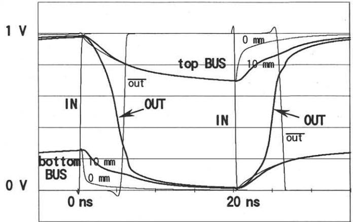
Fig.2 Simulated wave forms of Split level BUS.
