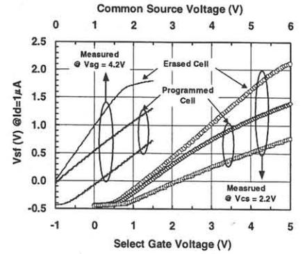
Fig. 3 Source-follower Voltage Vsf vs. select gate voltage  $V_{sg}$  and Vsf vs. common source voltage  $V_{cs}$  for Erased and Programmed cells.
