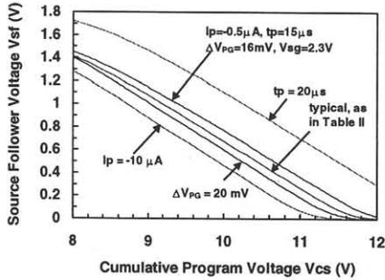
Fig. 7 Cumulative  $V_{cs}$  program characteristics of a SSI Flash cell programmed with varieties of program parameters.
