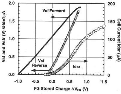
Fig. 1 Simulation results showing the Vsf read, Vsf (Reverse) read and Cell current Idsr read as a function of  $\Delta V_{FG}$  of the SSI Flash cell
