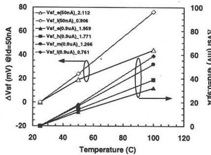
Fig. 11 Vsf dependence of temperature:  $\Delta V_{sf} = V_{sf} - V_{sf} @ 25C$  for erased (e), high (h), median (m) and low (l) cells (the Vsf values are included as last parts of the legend).
