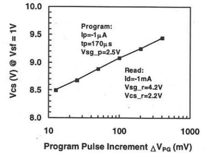
Fig. 9  $\Delta V_{PG}$  (program voltage pulse increment) dependence of cumulative program:  $V_{cs}$  @  $V_{sf} = 1V$  vs.  $\Delta V_{PG}$ .
