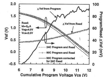
Fig. 12 Cumulative program dependence of temperature:  $V_{sf}$ - $V_{cs}$  curves generated @ 24C and @ 90C and  $V_{sf}$ - $V_{cs}$  @ 90C with read correction.  $\Delta V_{sf}$  from Read and from Program are shown.
