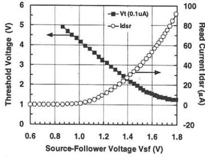
Fig. 2 Source-follower Vsf read ( $I_d = 1\mu A$ ) mapping to Cell threshold voltage  $V_t$  and Cell current Idsr measurements of the SSI Flash cell.
