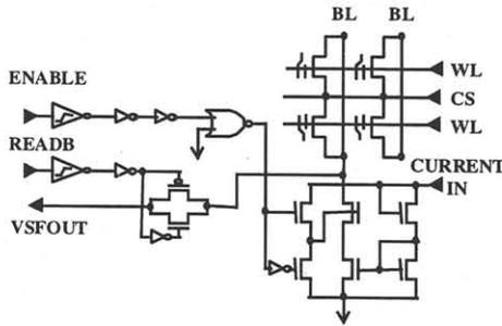
Fig. 4 Schematics showing the column driver circuit controlling the Read and the Program operations of the Flash memory array.
