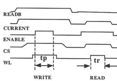
Fig. 5 Timing diagram showing the control signals and the pulses for Read and Program.
