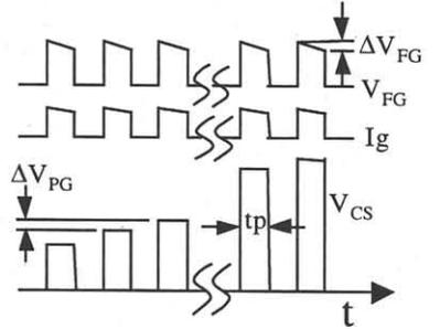
Fig. 6 A depiction of  $V_{cs}$  ( $=V_{PG}$ ),  $I_g$  and  $V_{FG}$  (FG voltage) as a function of time in the iterative programming sequence.
