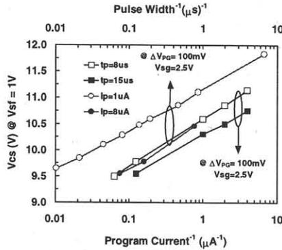
Fig. 8  $I_p$  (program current) and  $t_p$  (program pulse width) dependence of cumulative program:  $V_{cs}$  @  $V_{sf} = 1V$  vs.  $I_p^{-1}$  (Lower axis) and vs.  $t_p^{-1}$ .
