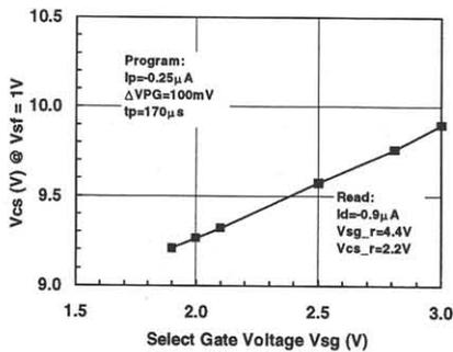
Fig. 10  $V_{sg}$  (select gate voltage) dependence of cumulative program:  $V_{cs}$  @  $V_{sf} = 1V$  vs.  $V_{sg}$ .
