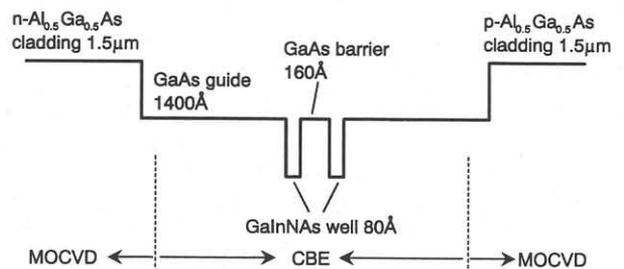
Fig. 1 Schematic structure of broad area GaInNAs/GaAs DQW laser. Schematic conduction band diagram is also shown.
