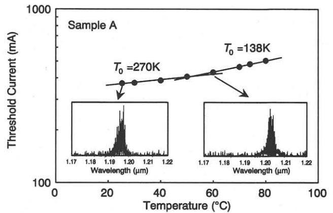
Fig. 3 Temperature dependence of threshold current of GaInNAs/GaAs laser diode.  $T_0$  of  $270\text{K}$  for  $25\text{-}50^\circ\text{C}$  and  $138\text{K}$  for  $50\text{-}80^\circ\text{C}$  were obtained. Inset figures show emission spectra at  $25$  and  $60^\circ\text{C}$ , respectively.
