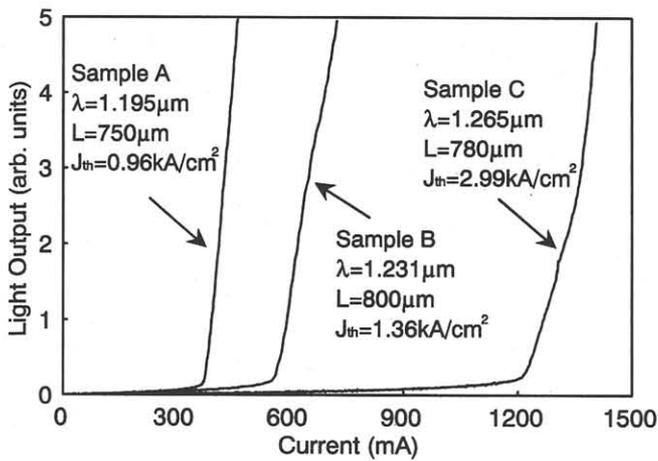
Fig. 2 L-I characteristics of GaInNAs/GaAs DQW lasers with three types of GaInNAs/GaAs DQW under pulsed condition.
