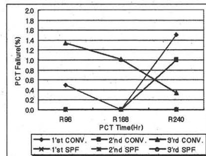
Fig. 11. The final PCT estimation graph of conventional fuse and SPF structures for three tries.
