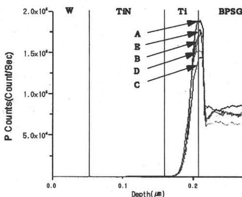
Fig. 6. The SIMS spectra of phosphorus concentration of the samples.
