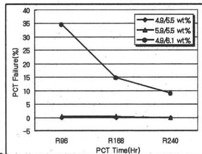
Fig. 8. The PCT estimation graph of boron and phosphorus concentration variation.
