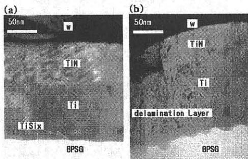
Fig. 4. TEM cross-section images of good and fail chips interface layer after PCT estimation.
