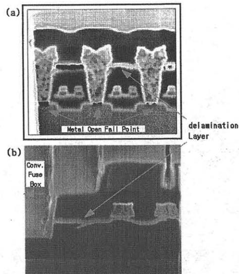
Fig. 3. Cross-sectional SEM of failure point by FIB.
