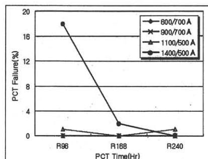
Fig. 9. The PCT estimation graph of barrier metal Ti/TiN thickness variation.
