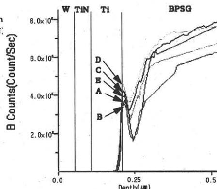
Fig. 5. The SIMS spectra of boron concentration of the samples.
