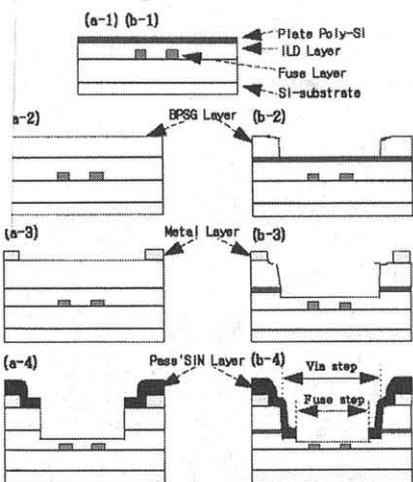
Fig. 1. The illustration of (a) the conventional fuse and (b) SPF process flow.
