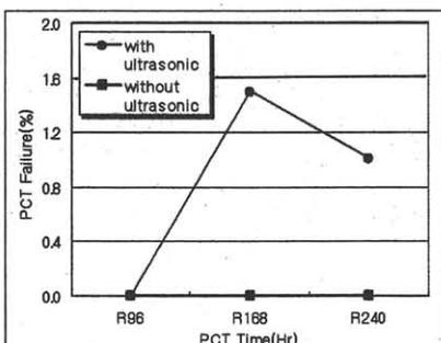
Fig. 10. The PCT estimation graph with or without ultrasonic agitation in cleaning.
