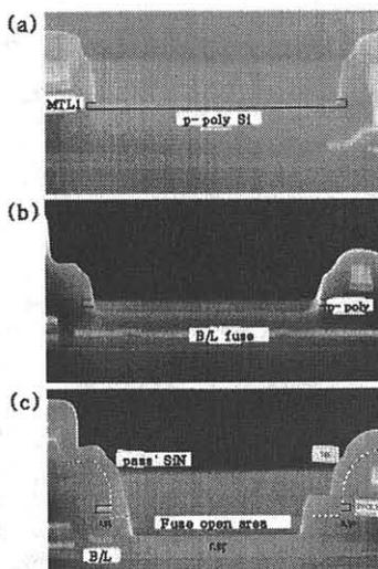
Fig. 2. Cross-sectional SEM photographs of process sequence for the SPF.
