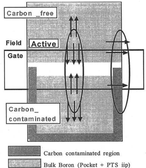
**Fig.6.** Schematic diagram showing the effect of carbon on the boron redistribution.
