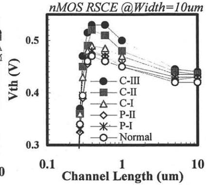
**Fig.4.** Threshold Voltage (Vth) as a function of Channel Length
