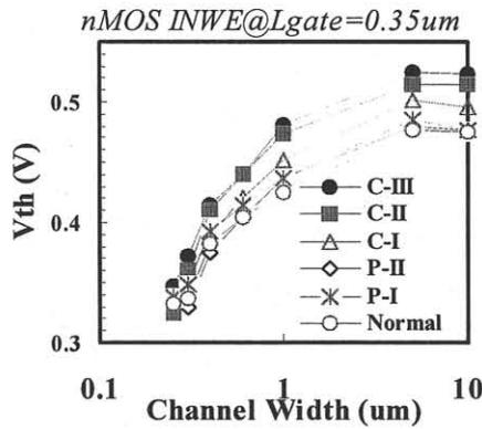
**Fig.3.** Threshold voltage as a function of channel width..
