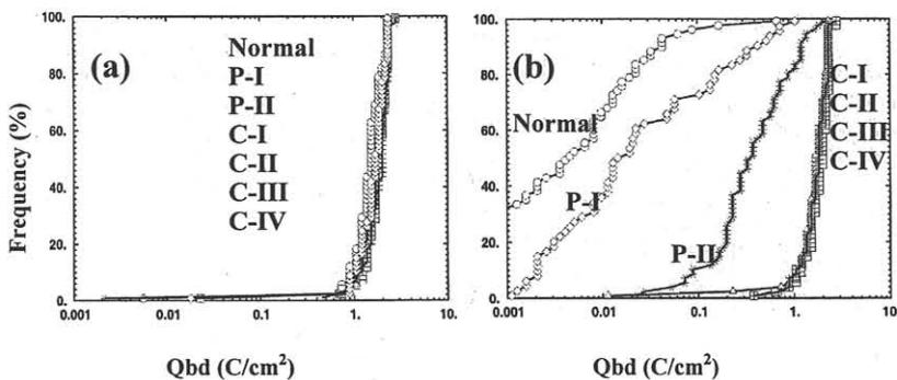
**Fig. 2.** N-MOS gate oxide Qbd characteristics. Test patterns are capacitor with gate poly overlap over trench edge (a) and over only active area (b).
