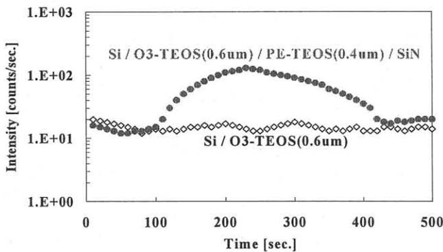
**Fig. 1.** Accelerated carbon contamination is detected at substrate under PE-TEOS by nitride capping followed by 1050 °C anneal for 1hr.
