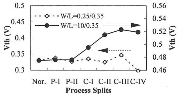
**Fig.5.** Threshold voltage as a function of process split.
