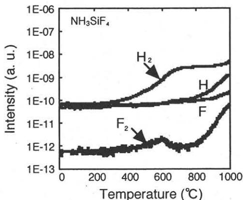
Fig.6 Thermal desorption mass spectroscopy (TDS) results of fluorinated  $\text{SiN}_x$  film formed employing  $\text{NH}_3/\text{SiF}_4$ .
