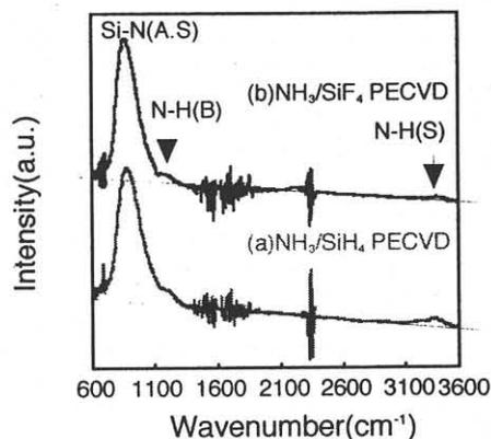
Fig.5 FT-IR spectra of (a)  $\text{SiN}_x$  film formed employing  $\text{NH}_3/\text{SiH}_4$  and (b) fluorinated  $\text{SiN}_x$  film formed employing  $\text{NH}_3/\text{SiF}_4$ .
