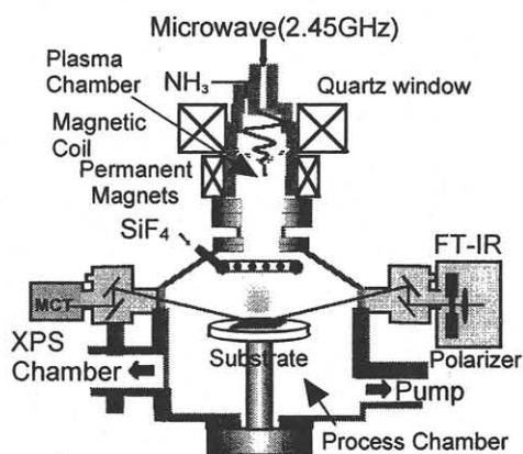
Fig.1 Schematic diagram of the experimental apparatus of typical ECR-PECVD system.
