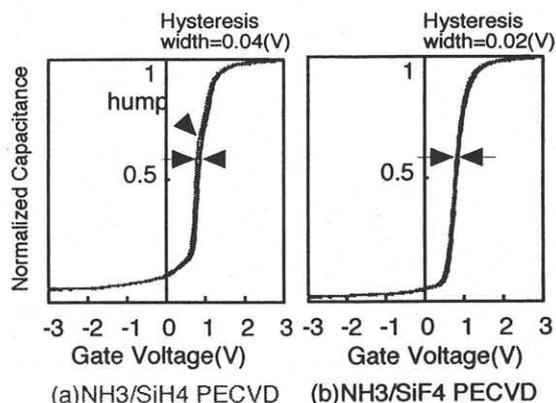
Fig.4 C-V curve of (a)  $\text{SiN}_x$  film formed employing  $\text{NH}_3/\text{SiH}_4$  and (b) fluorinated  $\text{SiN}_x$  film formed employing  $\text{NH}_3/\text{SiF}_4$ .
