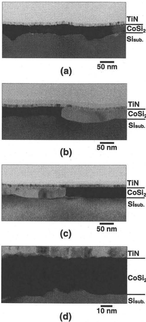
Fig. 1: Cross-sectional TEM photographs of  $\text{CoSi}_2/\text{p}^+\text{Si}(100)$ . The initial thickness of the TiN and the Co is 10 nm. The substrate is  $\text{p}^+\text{Si}(100)$  ( $B^+$  5kV 5e15/cm<sup>2</sup>, RTA 1000°C, 10 s). Pre-deposition wet-treatment solutions are (a) 0.6 % HF, (b) BHF, and (c) amonium-sulphate-added BHF. A typical magnified image of the faceting grain of  $\text{CoSi}_2(100)//\text{Si}(100)$  is shown in (d).
