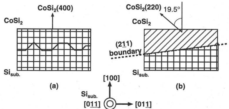
Fig. 3: Epitaxially grown grain models determined from TEM and XRD results: (a)  $\text{CoSi}_2(100)//\text{Si}(100)$  model; (b)  $(211)\text{-}\Sigma 3$ -twin model
