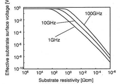
**Fig.4** Effective rms substrate voltage for evaluation of cross-talk interference.
