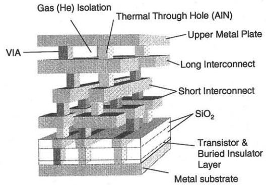
**Fig.8** Schematic view of gas-isolated interconnect, metal substrate structure.
