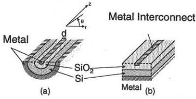
**Fig.1** (a) Stacked coaxial structure in this study
