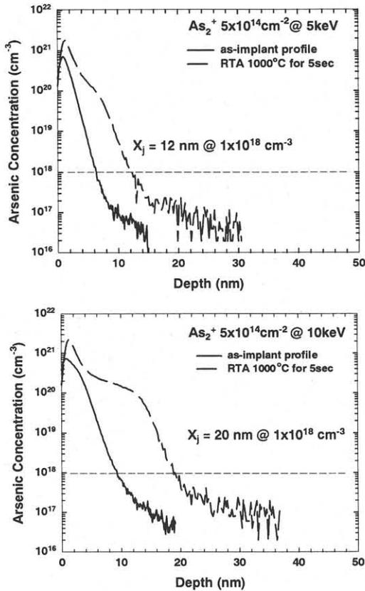
Fig. 2. As-implanted and post-RTA SIMS profiles of arsenic. Because SIMS analysis for as-implanted arsenic profiles was carried out without screen oxide strip, an arsenic concentration at silicon surface regions was measured with the small transient error of SIMS measurement system.
