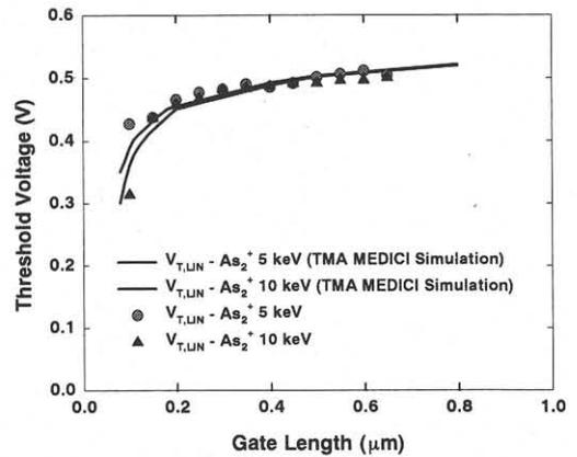
Fig. 6. The improved threshold voltage roll-off characteristics are achieved in the As<sub>2</sub><sup>+</sup> 5 keV NMOSFETs.
