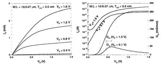
Fig. 5. The ID-VG and ID-VD characteristics of fabricated NMOSFETs with gate length of 70 nm.
