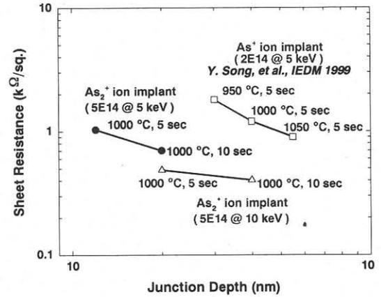
Fig. 4. Sheet resistance versus junction depth for As ion implantation process.
