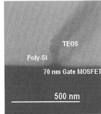
Fig. 3. The cross-sectional SEM photographs of 70 nm gate length NMOSFET
