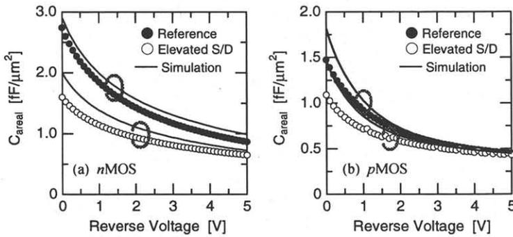
Fig. 4 Junction capacitance dependence on reverse drain voltage, (a) *n*MOS, (b) *p*MOS.
