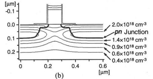
Fig. 3 Simulated B profiles and *pn* junction boundary (*n*MOS), (a) Elevated S/D, (b) Reference.
