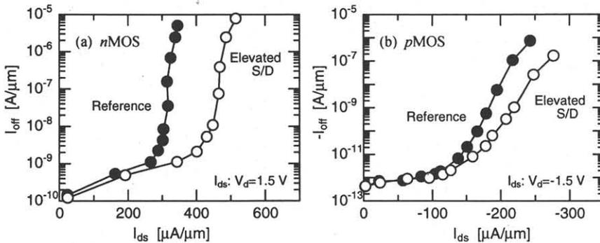
Fig. 7  $I_{on}$ - $I_{off}$  characteristics, (a) *n*MOS, (b) *p*MOS.
