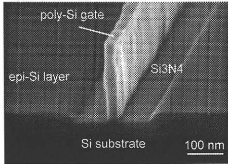
Fig. 2 Cross sectional SEM image of the elevated S/D transistor.
