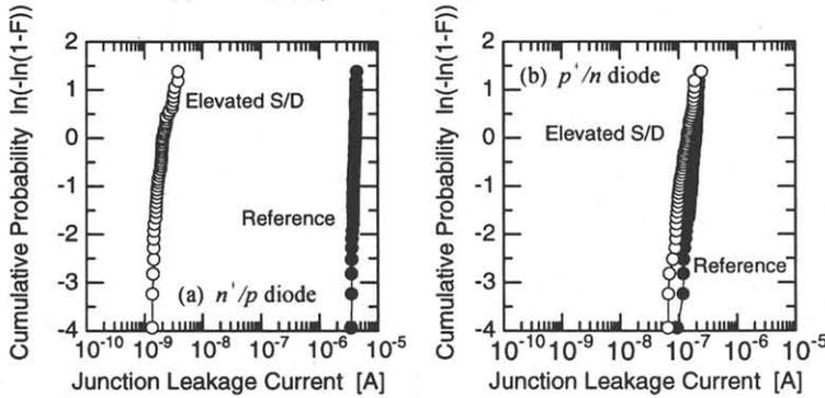
Fig. 5 Junction leakage characteristics, (a) *n*MOS, (b) *p*MOS.
