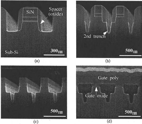
Fig. 2 The process flow of T-shaped STI. (a) active definition and spacer formation (b) 2nd trench etch, (c) spacer wet stripped, (d) after trench filling, CMP, gate-poly deposition.
