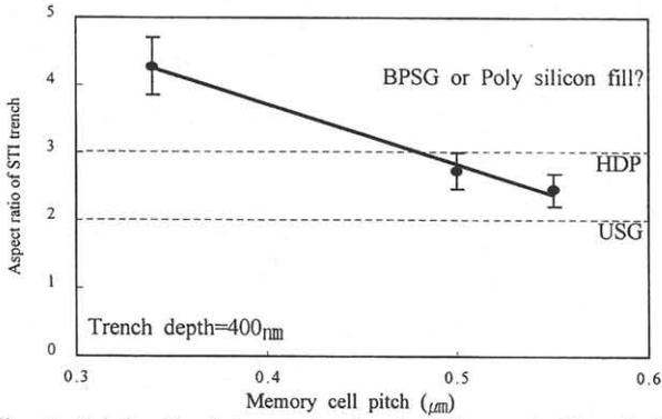
Fig. 1 Relationship between the trench filling material and the aspect ratio according to device scale down. Dotted lines are limitations of gapfill with HDP and USG.
