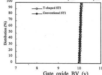
Fig. 9 PMOS Gox BV distributions at  $I_g=1\mu\text{A}$  (Area= $400*250\mu\text{m}^2$ ).
