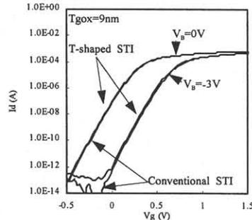
Fig. 8  $I_g$ - $V_g$  characteristics of NMOSFETs with  $W=20\mu\text{m}$ ,  $L=0.5\mu\text{m}$ .
