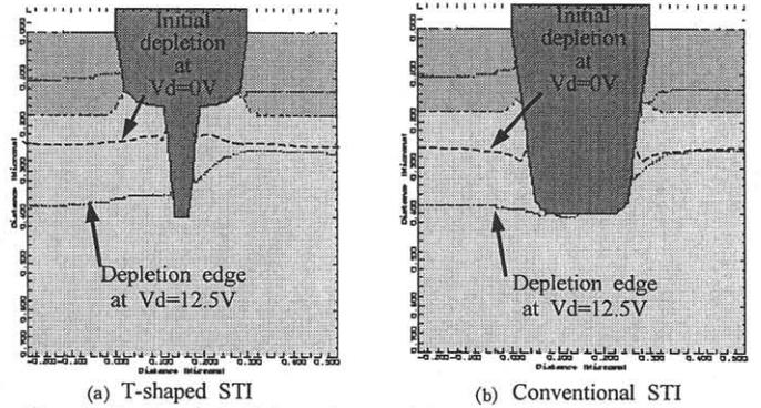
Fig. 6 Simulated depletion characteristics according to drain voltage. Because of T-shaped trench profile, T-shaped STI shows narrow depletion width than conventional STI.
