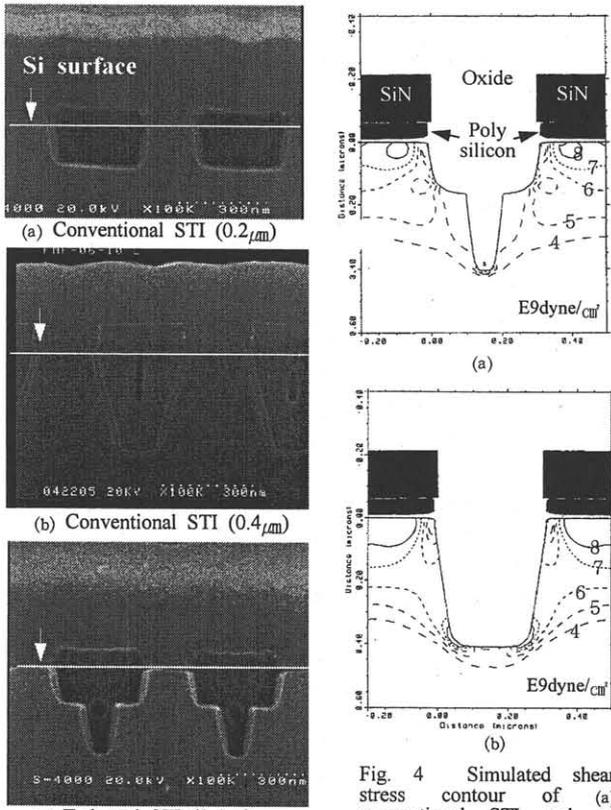
Fig. 4 Simulated shear stress contour of (a) conventional STI and (b) T-shaped STI.
