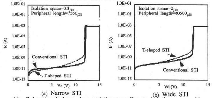
Fig. 7 Junction leakage characteristics according to isolation space with T-shaped STI and conventional STI.
