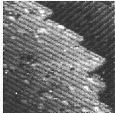
Fig. 1 STM image of a Si(100)-2x1 clean surface. The image was obtained at a sample bias of +2.0 V. The scan area was 20 nm x 20 nm.
