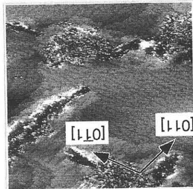
Fig. 4 STM image of a Si surface after exposing to radical nitrogen of about 50 L at 850°C. The image was obtained at a sample bias of +4.0 V. The scan area was 100 nm x 100 nm.
