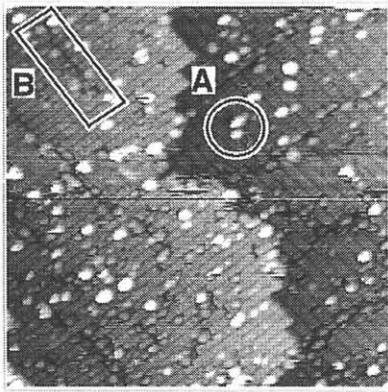
Fig. 2 (a) STM image of a Si surface after exposing to radical nitrogen of about 1 L at 850°C. The image was obtained at a sample bias of +2.0 V. The scan area was 25 nm x 25 nm.
