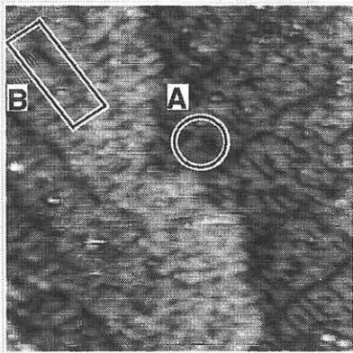
Fig. 2 (b) STM image of a Si surface after exposing to radical nitrogen of about 1 L at 850°C. The image was obtained at a sample bias of -2.0 V. The scan area was 25 nm x 25 nm.
