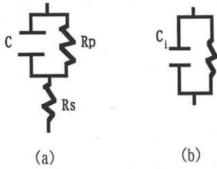
Fig. 1 Equivalent circuit models.
