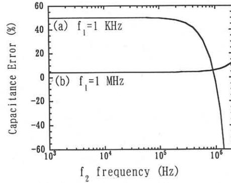
Fig. 2 Error (%) of calculated capacitance vs  $f_2$ .  $f_1$  is 1kHz in (a) and 1MHz in (b).
