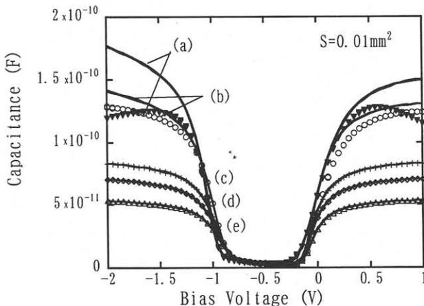
Fig. 6 C-V characteristics of nMOSFET devices with oxide layer thickness of (a) 1.8nm (b) 2.5nm (c) 3.6nm (d) 4.6nm (e) 6.2nm measured at a fixed frequency are indicated by symbols. Calculated capacitance is indicated by continuous lines.
