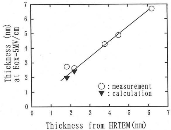
Fig. 7 Comparison of oxide thickness obtained from single-frequency measurement (O), and two-frequency calculations (V) and HRTEM observations.
