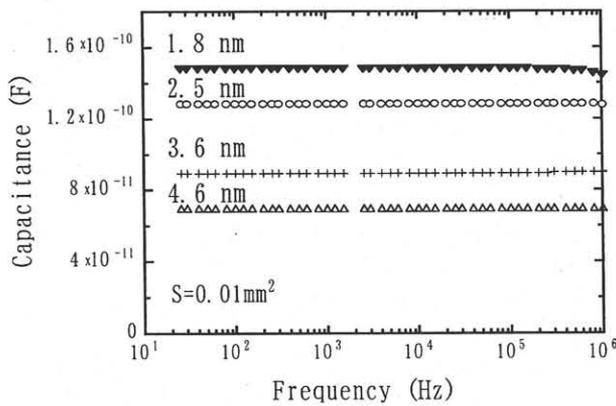
Fig. 4 Frequency dependence of capacitance for various oxide layer thicknesses at a bias of -2V.
