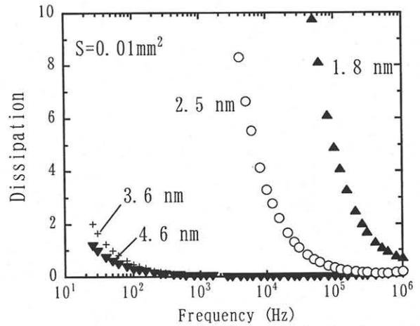
Fig. 5 Frequency dependence of dissipation values for various oxide layer thicknesses at a bias of -2V.
