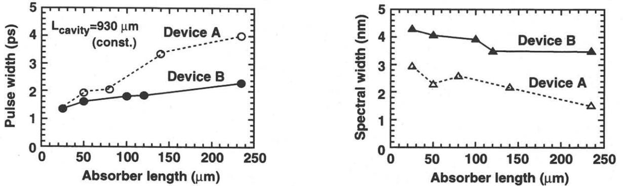
Fig. 2 Dependence of the pulse widths and spectral widths on the absorber length of 930- $\mu$ m end-absorber PML-LDs
