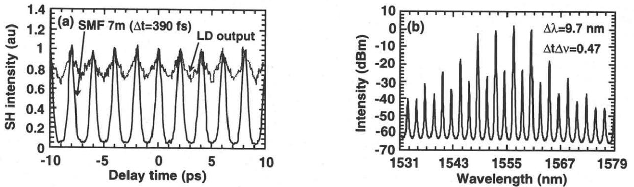
Fig. 4 (a) SHG correlation traces and (b) optical spectrum of a 500 GHz optical pulse train generated from a 170- $\mu$ m GRIN-SCH CPM-LD
