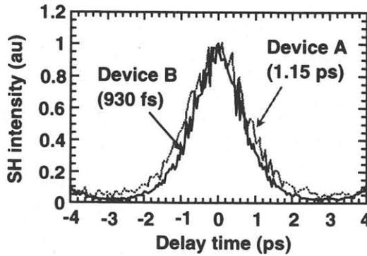
Fig. 3 Comparison of the SHG correlation traces of 160 GHz CPM-LDs
