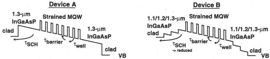
Fig. 1 Band diagrams of two types of PML-LDs used in this work
