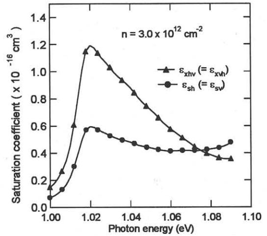
Fig. 2 Self- and Cross-saturation of QW VCSEL
