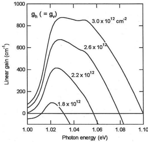
Fig. 1 Linear gain of QW VCSEL at 300 K.
