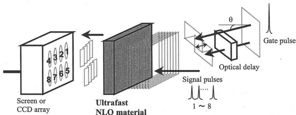
Fig.1. Schematic diagram of the serial-to-parallel pulse conversion system.
