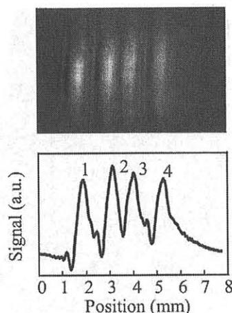
Fig.3. Output signals and intensity profile of the CCD differential image using a SQ J-aggregate film.
