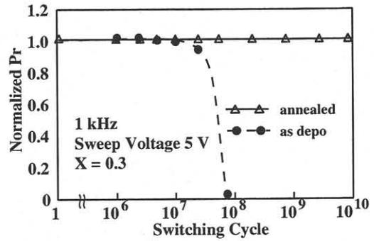
Fig.4. Fatigue properties of as-deposited and annealed STN films.
