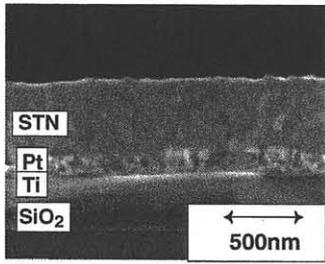
Fig.2. Cross sectional view of STN film.
