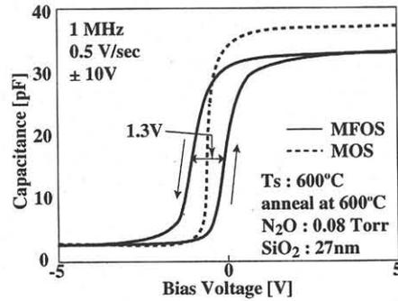
Fig.5. C-V characteristics of MFOS and MOS structures.
