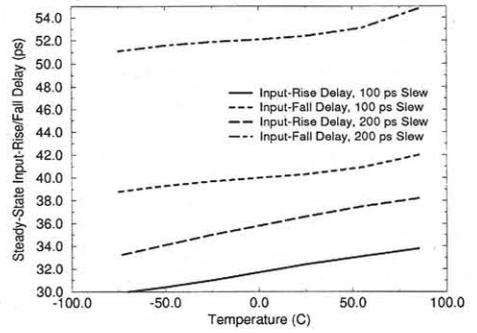
Fig.3: First 'input-rise' delays and first 'input-fall' delays for an inverter as a function of temperature for two initial conditions (inverter input initially a LOW or at HIGH)
