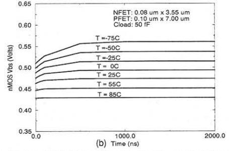
Fig.1: (a) Input-rise delays, (b) nMOS body voltages before input-rising transitions as functions of time and temperature for an inverter. Inverter input is initially at LOW and then continuously switches at 1GHz with 50% duty cycle and 100ps slew.
