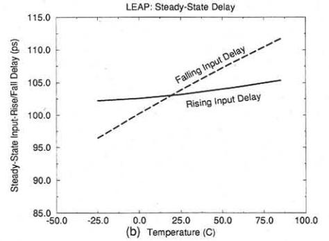
Fig.6: (a) First 'input-rise' delays and first 'input-fall' delays (b) steady-state 'input-rise' delay and 'input-fall' delay as functions of temperature for LEAP circuit.
