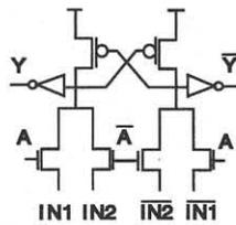
Schematic of a cross-coupled dual-rail CPL circuit
