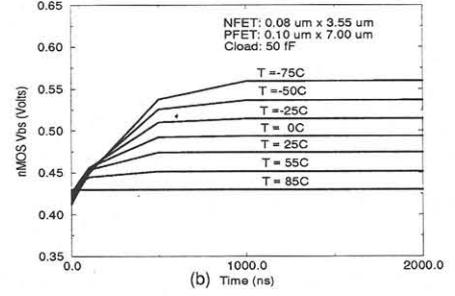
Fig.2: (a) Input-rise delays, (b) nMOS body voltages before input-rising transitions as functions of time and temperature for an inverter. Inverter input is initially at HIGH and then continuously switches at 1GHz with 50% duty cycle and 100ps slew.
