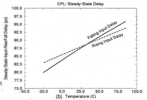
Fig.7: (a) First 'input-rise' delays and first 'input-fall' delays (b) steady-state 'input-rise' delay and 'input-fall' delay as functions of temperature for CPL circuit.
