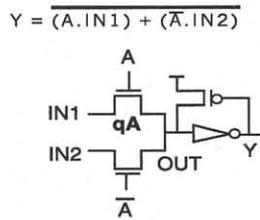
Schematic of a single-ended LEAP circuit
