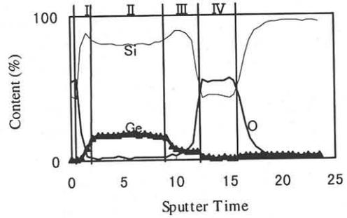
Fig.5 Depth profiling of Ge and O in the SiGe double layer structure measured by AES.
