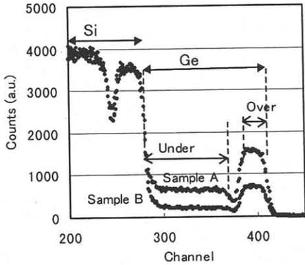
Fig. 2 RBS spectrum from each sample.
