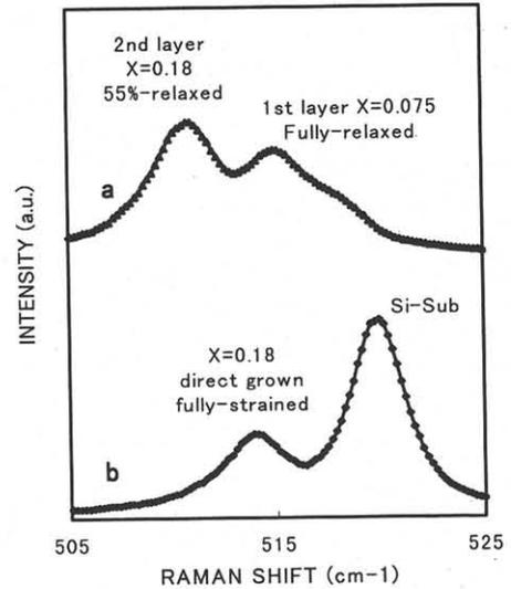
Fig.7 RAMAN spectrum from the SiGe double layer structure (a) and the conventional structure (b).
