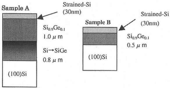
Fig. 1 Schematic illustration for two samples to evaluate the Ge diffusion.
