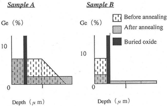
Fig. 3 Schematic illustration for Ge diffusion during annealing.
