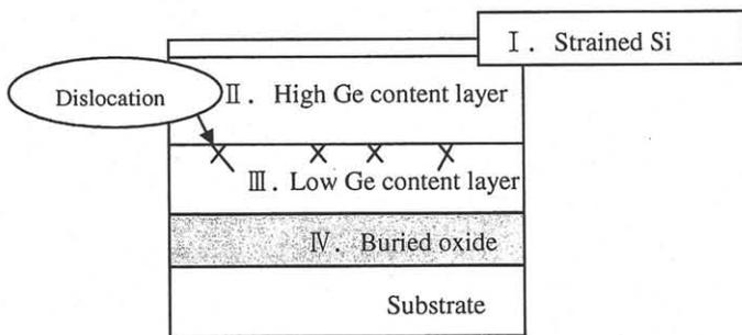
Fig. 4 Schematic illustration of SiGe double layer structure.
