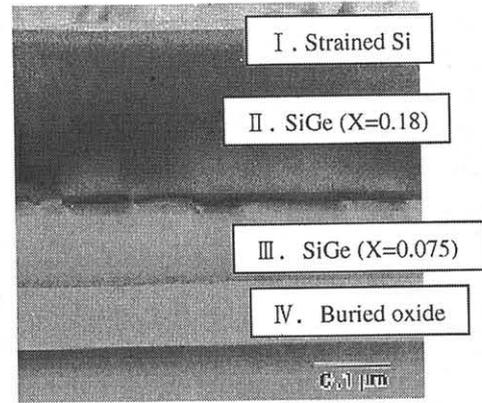
Fig.6 Cross-sectional TEM image of the double layer structure.
