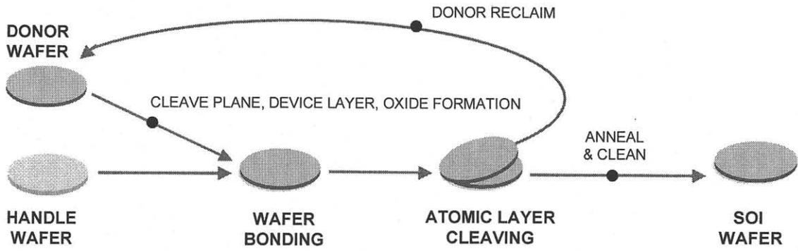
Figure 1. Nanocleave™ process flow.
