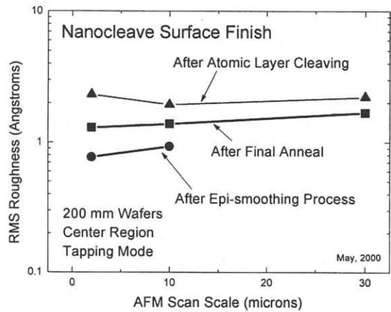
Figure 3. AFM measurements of Si roughness after cleaving, after final anneal and after an epi-
