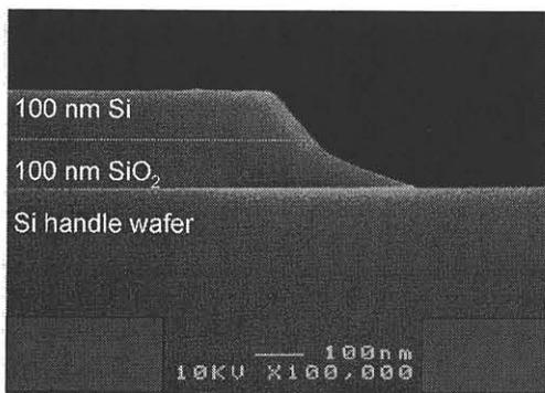
Figure 4. SEM cross-section view of the SOI edge taper for a 100 nm Si(110) layer on a 100 nm BOX.
