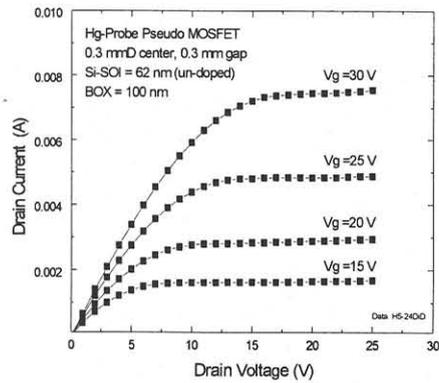
Figure 5. Hg-probe pseudo-MOSFET characteristics of an SOI wafer with Si-SOI thickness of 62 nm and a BOX of 100 nm.
