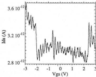
Fig. 3 Gate conductance oscillations with  $V_{ds}=48$  mV.
