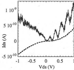
Fig. 2 Current-voltage plot of oxidized SET (dotted line) at 4.2 K, channel width of 60 nm.  $dI/dV$  (solid line) depicting step-like structures.
