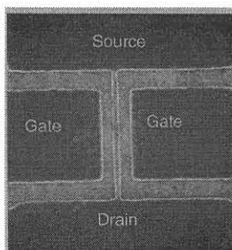
Figure 1 A scanning electron micrograph of a fabricated device. There are two side gates separated from the channel by 120 nm.
