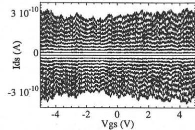
Fig. 5 Gate conductance oscillations of annealed SET with  $V_{ds} = -20$  mV to 20 mV in steps of 2 mV.
