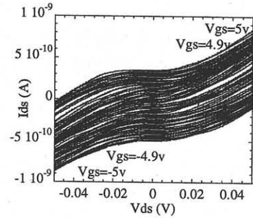
Fig. 4 Current-voltage characteristics of annealed SET with gate sweep from -5 V to 5 V. Measurement performed at 4.2 K.
