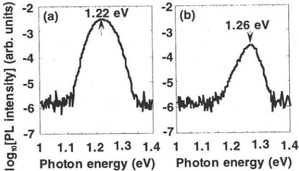
Fig. 4 PL from InAs SAQDs (a) and GaSb ML QW (b). Spectra of (a), and (b) were obtained from independent samples.
