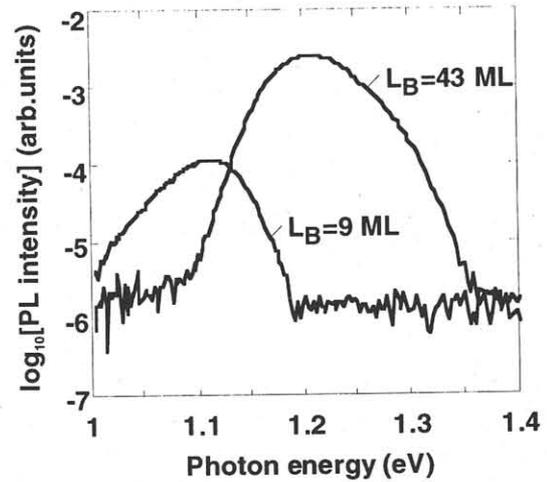
Fig. 5 PL spectra of InAs SAQDs coupled with GaSb ML QW having GaAs barrier thickness of 43 ML and 9 ML, respectively, at 77K.
