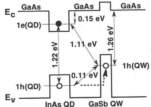
Fig. 6 The obtained schematic band diagram of InAs SAQDs coupled with GaSb ML QW.
