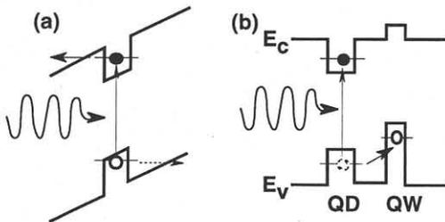
Fig. 1 Schematic band diagram of a biased InAs QD (a) and a QD coupled type II QW (b).
