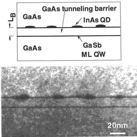
Fig. 3 Cross-sectional TEM image of InAs SAQDs coupled with GaSb ML QW. GaAs barrier thickness of  $L_B$  was 43 ML. Schematic sample structure is also shown.
