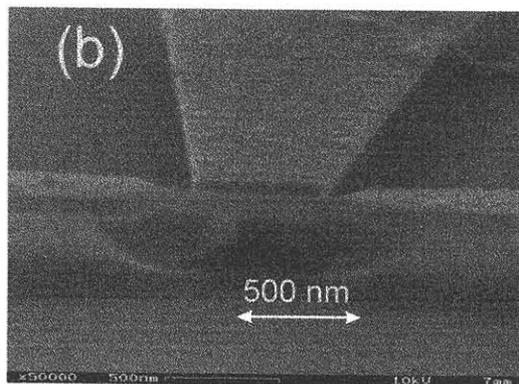
Fig. 1(a) Shown is a top view and in (b) a side view of the suspended silicon nanowire used here. The strongly doped wire is clearly underetched, the gate allows to tune the carrier density in the wire. The dimensions are:  $700 \times 24 \times 80 \text{ nm}^3$  (length  $\times$  width  $\times$  thickness).
