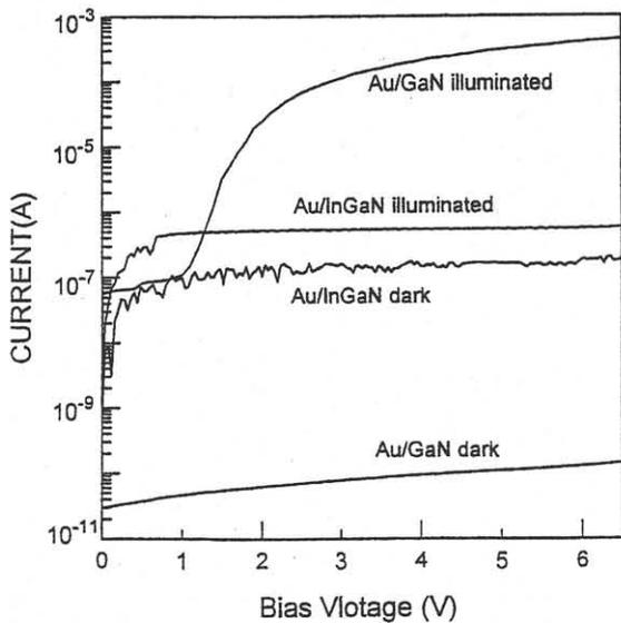
Fig.2 Dark and illuminated current-voltage characteristics of n-GaN and n-In<sub>0.2</sub>Ga<sub>0.8</sub>N MSM photodetectors, respectively, with Schottky contact metals of Au.
