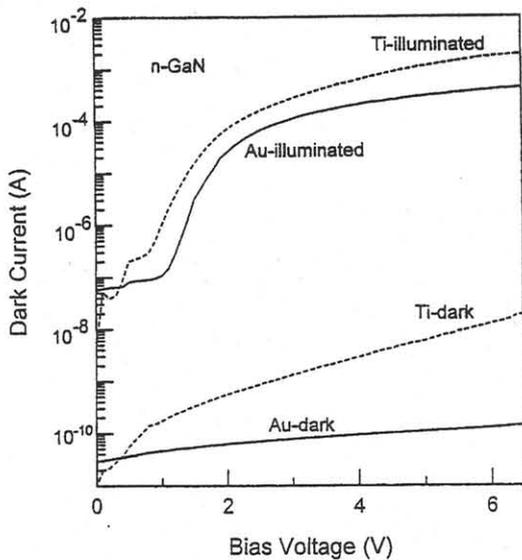
Fig.1 Dark and illuminated current-voltage characteristics of n-GaN MSM photodetectors with Schottky contact metals of Au and Ti, respectively.
