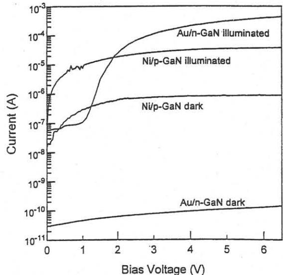
Fig.5 Dark and illuminated current-voltage characteristics of Au/n-GaN and Ni/p-GaN MSM photodetectors, respectively.
