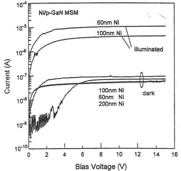
Fig.4 Dark and illuminated current-voltage characteristics of Ni/p-GaN MSM photodetectors with different Schottky contact thicknesses.
