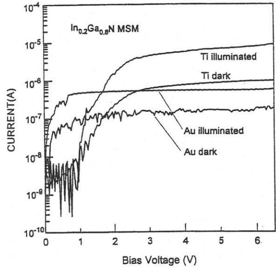
Fig.3 Dark and illuminated current-voltage characteristics of n-In<sub>0.2</sub>Ga<sub>0.8</sub>N MSM photodetectors with different Schottky contact metals of Au and Ti, respectively.
