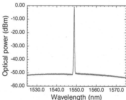
Fig. 3 Oscillation spectrum at 25°C, 60 mA
