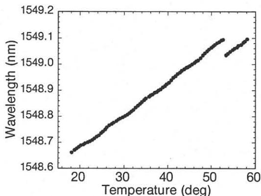
Fig. 5 Oscillation wavelength against temperature with APC
