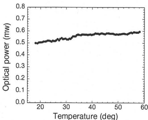
Fig. 4 Optical power against temperature with APC
