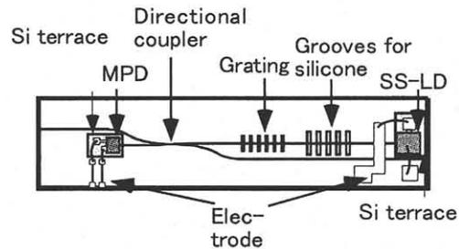
Fig. 1 Configuration of proposed external cavity laser
