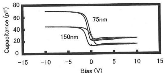
Fig.6 C-V characteristics of BLT films with different thicknesses.
