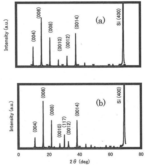
Fig.3 XRD patterns of BLT films. (a) c-axis orientation (b) random orientation
