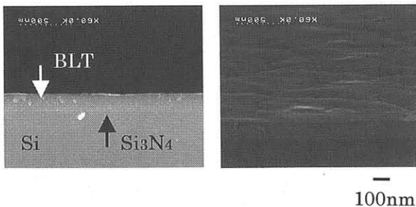
Fig.2 Surface morphology of BLT film on Si<sub>3</sub>N<sub>4</sub>
