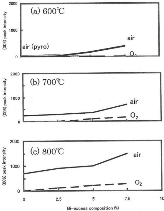
Fig.1 Relationships between Bi-excess composition and XRD (006) peak intensity. (a)600°C (b)700°C (c)800°C
