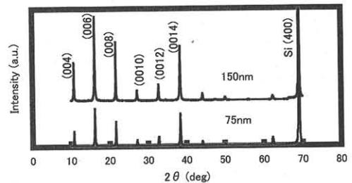
Fig.5 XRD patterns of BLT films with different thicknesses.
