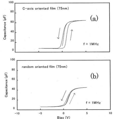
Fig.4 C-V characteristics of BLT diodes. (a) c-axis orientation (b) random orientation
