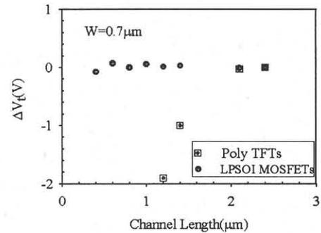
Fig. 6.  $V_t$  roll-off of LPSOI MOSFET and poly TFTs
