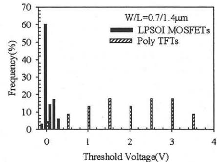
Fig. 7. Uniformity of the threshold voltage across a wafer for poly TFTs and LPSOI MOSFETs
