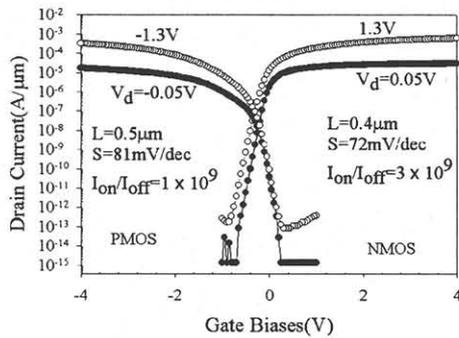
Fig. 2. Subthreshold characteristics of n-channel and p-channel LPSOI MOSFETs.
