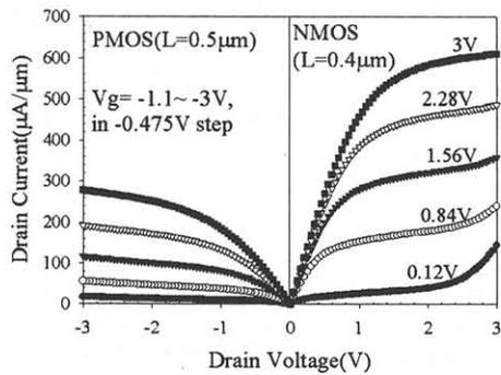
Fig. 3.  $I_d$ - $V_d$  of LPSOI NMOSFET and PMOSFET
