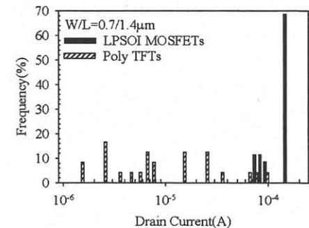
Fig. 8. Distribution of  $I_D$  ( $V_d=2V$ ,  $V_g=3V$ ) across a wafer for poly TFTs and LPSOI MOSFETs
