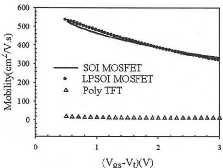
Fig. 4. Mobility vs.  $V_g$ - $V_t$  of a SOI MOSFET, LPSOI MOSFET and a polysilicon TFT at  $V_{ds}=0.05V$
