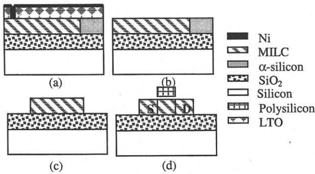
Fig. 1. Key steps for the formation of large grain poly-Si and LPSOI MOSFET fabrication.
