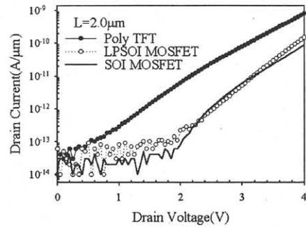
Fig. 5. GIDL characteristics for a poly TFT, LPSOI MOSFET and a SOI MOSFET
