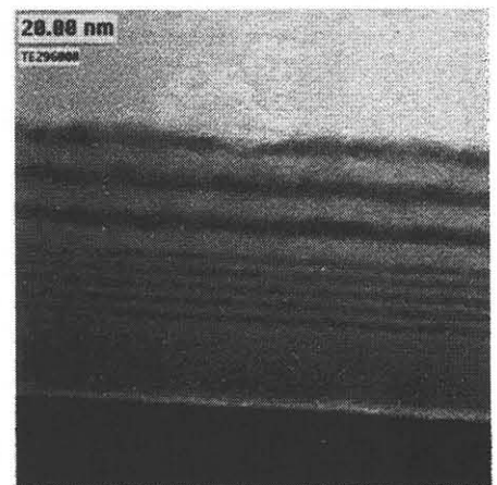
Fig. 5. TEM micrograph of nanolaminate dielectrics grown by ALD technique.
