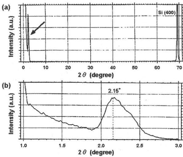
Fig. 2 X-ray diffraction patterns of mesoporous silicate glass film deposited on Si substrate. (a) A sharp peak of mesoporous silica is marked by solid arrow. The marked XRD peak is shown in detail in (B).
