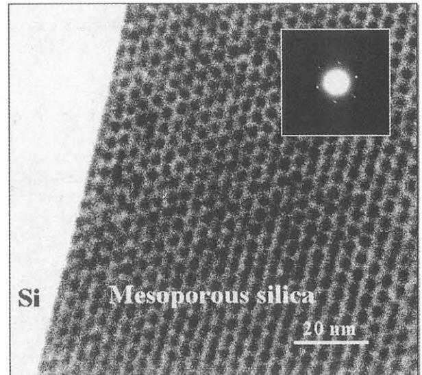
Fig. 3 Cross-sectional TEM photograph of mesoporous silicate glass film deposited on Si substrate. ED pattern is also inserted in this figure.
