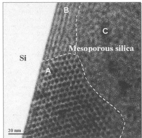
Fig. 4 Cross-sectional TEM photograph revealing domains (white broken lines are guided for eyes) of mesoporous silicate glass film deposited on Si substrate.
