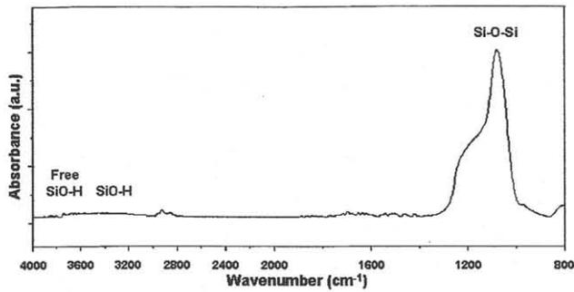
Fig. 1 FT-IR spectrum of mesoporous silicate glass film deposited on Si substrate.
