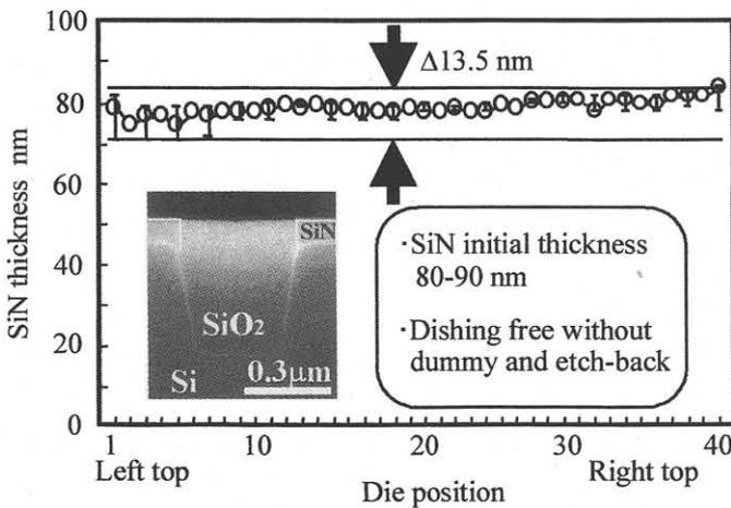
Fig. 5 Within wafer non-uniformity by applying FX-CMP to STI planarization.
