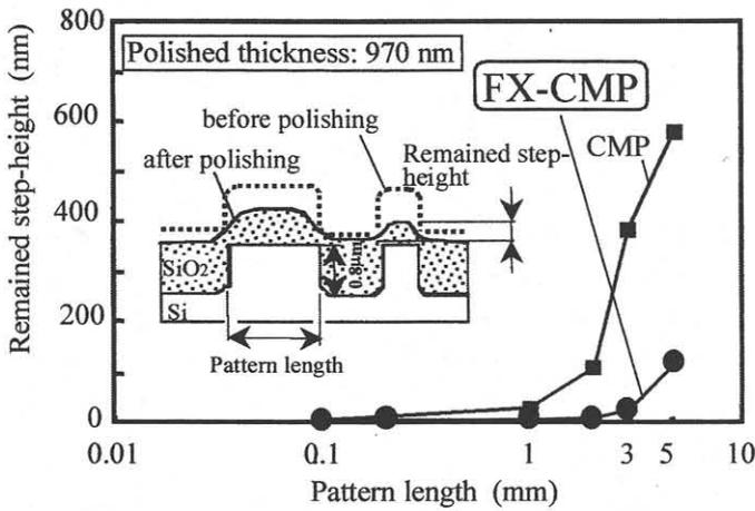
Fig. 3 Degree of planarization characteristics between FX-CMP and CMP.
