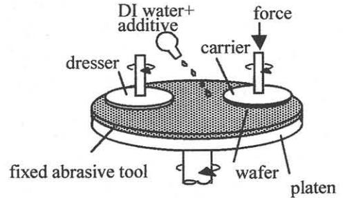
Fig. 2 Schematics of FX-CMP system.
