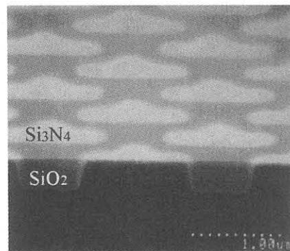
Fig. 6 Cross-sectional SEM photograph of 0.3-μm-node-test patterns after STI planarization.
