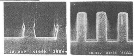
Fig.3 SEM image of gate profile due to gate etch method. The improvement in degree of anisotropy was obtained by TM bias. (a) Type I (b) Type II
