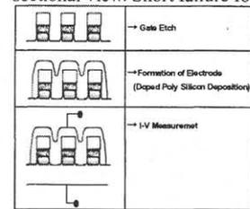
Fig.6 To verify gate edge damage, oxide leakage was measured using fabricated electrode just after gate etch. Device with Type II shows the larger degradation when compared to that with type I.
