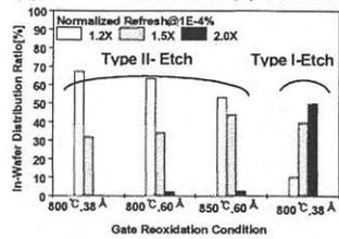
Fig.9 Significantly deteriorated tail component could not be recovered even after re-oxidation process.
