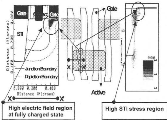
Fig.1 When defect is at the drain just below gate edge under the influence of high field and high STI stress, the deterioration of tail component in retention time become extremely severe.
