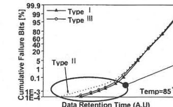
Fig.13 Device with Type III has a comparable tail component of retention time when compared to the device with Type I. (a) Cumulative retention time (b) Distribution ratio of tail component of retention time in wafer.
