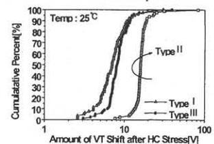
Fig.12 VT shift due to the localization of trapped hot carriers near the drain region.
