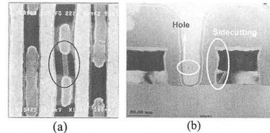
Fig.4 Short failure between storage node plug due to BPSG void filled with plug Poly-Si due to gate etch method was observed for device employing Type I etch method. (a) Top-view (b) Cross sectional view. Short failure for device employing Type II was not observed in (c)
