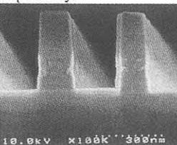
Fig.10 Device with Type III represents a comparable etch profile to device with Type II
