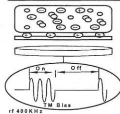
Fig.2 Schematic concept of TM bias in ECR plasma etching system.
