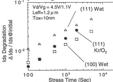
Fig.8 Stress-time dependence of Hot-carrier-induced Ids degradation for NMOS FETs fabricated by (100) Wet 700°C, (111) Wet 700°C, and (111) Kr/O<sub>2</sub> 400°C oxidation.
