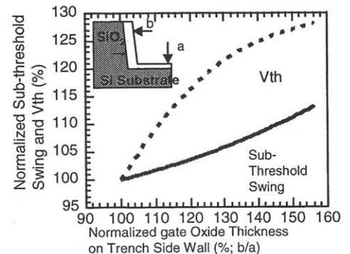
Fig.7 Simulated Id and sub-threshold swing improvement by gate oxide thickness control at side wall of trench. Bottom oxide thickness is 16nm .
