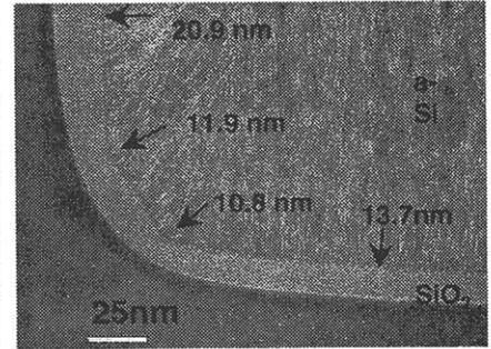
Fig.5 Cross sectional TEM view of 14nm thick oxide grown by dry O<sub>2</sub> 900 °C inside trench.
