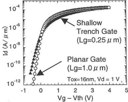
Fig.6 Id - Vg characteristics of the trench MOS FET and planar MOS FET with thermally formed gate oxide.
