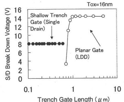
Fig.9 Vth and S/D breakdown voltage roll-off by gate length of trench gate and planar NMOS FET, both by thermal gate oxidation. S/D breakdown voltage at the trench gate is limited by drain to sub breakdown.
