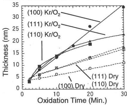
Fig.2 Dependence of oxidation rate of Kr/O<sub>2</sub> plasma 400°C and dry O<sub>2</sub> 900°C on Si surface orientation.
